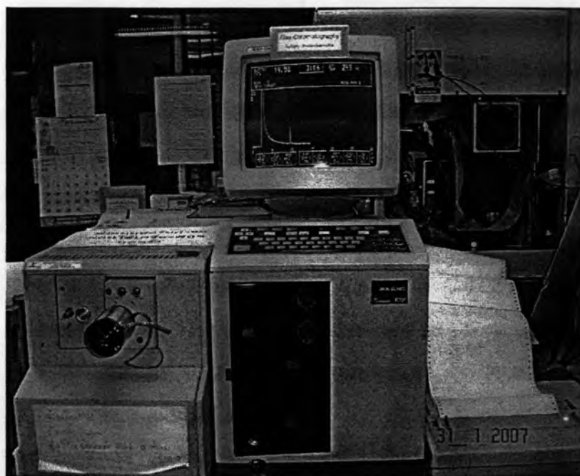
Figure 3.2 Gas chromatograph for analysis of methyl ester
