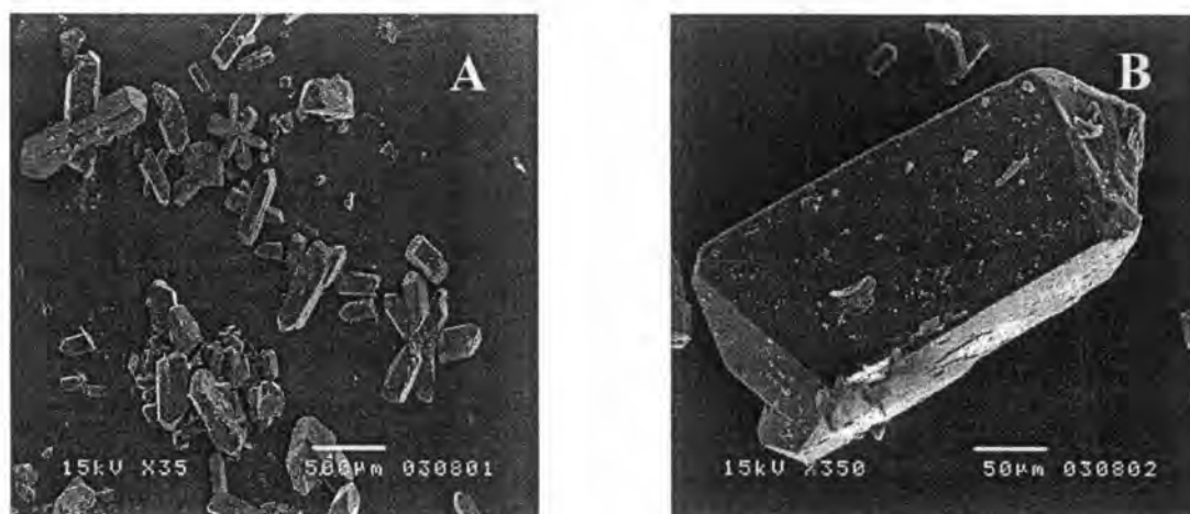
Figure 3.2 Scanning electron photomicrographs of BDM crystals (A-magnification of 35 and B-magnification of 350)
