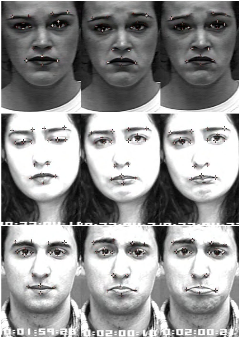
Figure 4.5: This figure shows tracking results of three image sequences that are labeled as sadness. Each row is for each image sequence. The first, the second, and the third columns are the first, the middle, and last frames of the image sequences, respectively.
