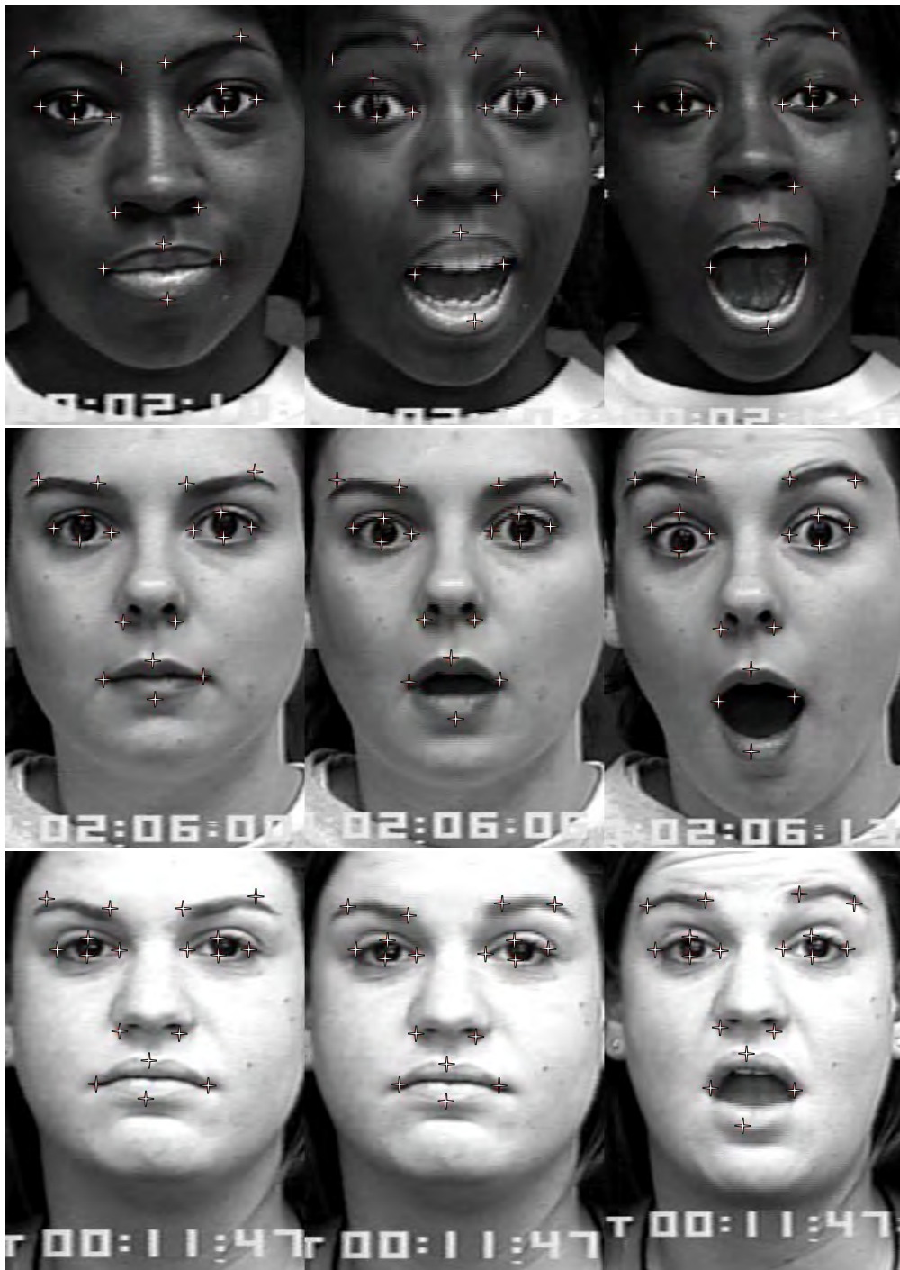
Figure 4.6: This figure shows tracking results of three image sequences that are labeled as surprise. Each row is for each image sequence. The first, the second, and the third columns are the first, the middle, and last frames of the image sequences, respectively.
