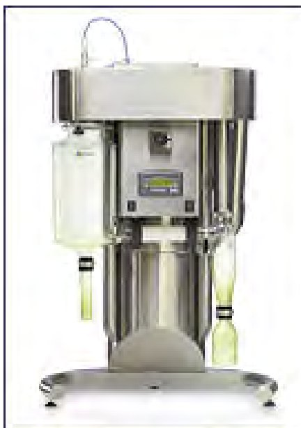
Figure 11 Spray dryer (Model SD-06, Labplant, Ltd., UK)
