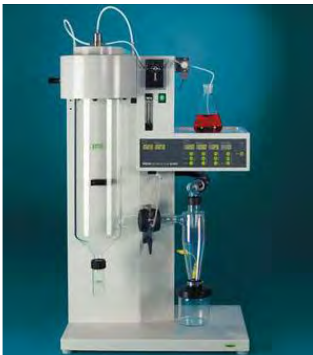
Figure 13 Spray dryer B-290 (Buchi Mini, Switzerland)
