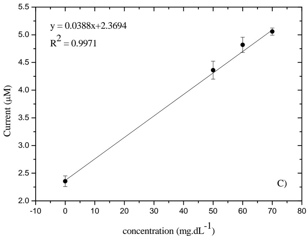
**Figure 4.14** The relationship between the peak current and the concentration of cholesterol in bovine serum. The concentrations of cholesterol in bovine serum are A) 20 mg·dL<sup>-1</sup>, B) 40 mg·dL<sup>-1</sup>, C) 60 mg·dL<sup>-1</sup>. Conditions: running buffer, a 40 mM PB buffer (pH 7.0) solution containing 0.68 U·mL<sup>-1</sup>, separation potential, +1600 V; injection potential, +450 V; time, 20 s; at 25 μm Au wire working electrode.
