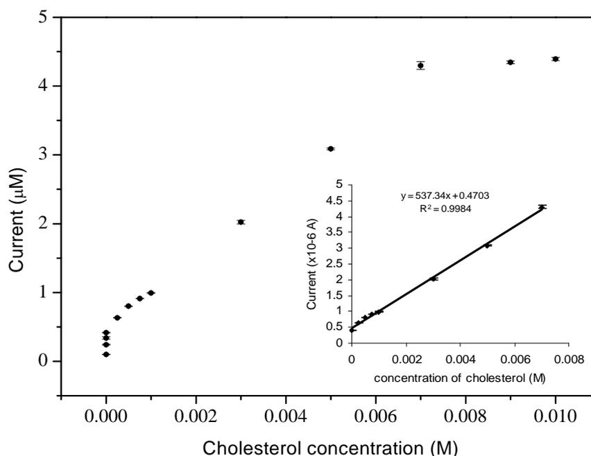
**Figure 4.13** The calibration curve of cholesterol and linear range is shown in the insert Conditions: running buffer, a 40 mM PB buffer (pH 7.0) solution containing  $0.68 \text{ U}\cdot\text{mL}^{-1}$ , separation potential, +1600 V; injection potential, +450 V; injection time, 20 s; at  $25 \mu\text{m}$  Au wire working electrode.
