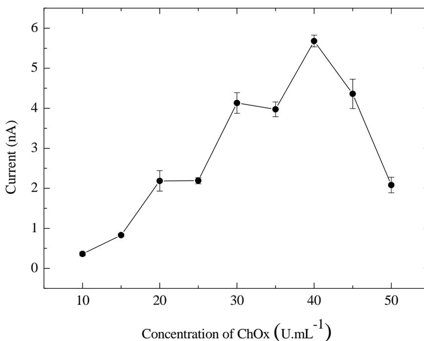
**Figure 4.3** The effect of running buffer concentration on peak current of -1 mM cholesterol. Conditions: running buffer, a PB buffer (pH 7.0) solution; detection potential, +0.5 V, separation potential, +1300 V; injection potential, +450 V; injection time, 20 s; at 25  $\mu\text{m}$  Au wire working electrode.
