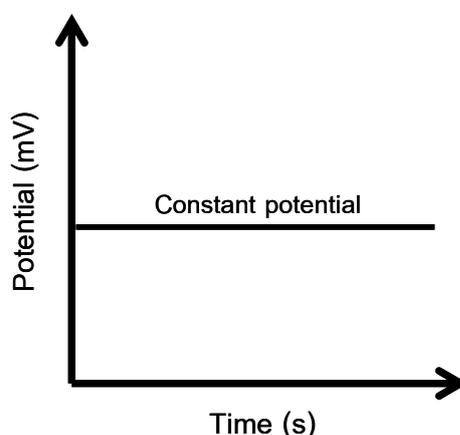
**Figure 2.8** A typical waveform employed in amperometry.
