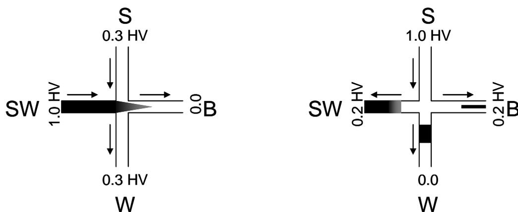
**Figure 2.14** Principle of pinched injection. Black stream is the sample, and white stream is the mobile phase. S: sample, SW: sample waste, B: buffer, and W: waste.
