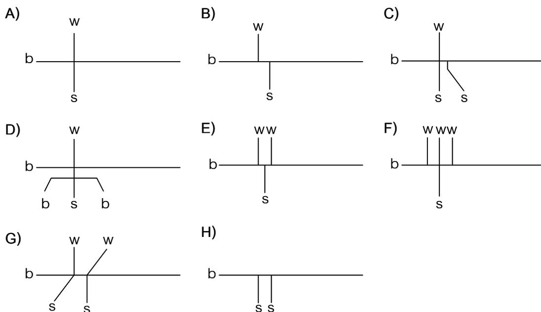
**Figure 2.12** Examples of sample injector types. A) cross, B) double-T, C) double-L, D) double cross, E) triple-T, F) multi-T, G) stacking type, and H)  $\pi$ -injector. Sample inlet s, waste w and BGE inlet b are indicated [20].
