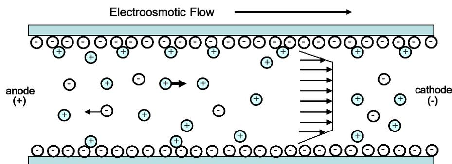
**Figure 2.4** Electroosmotic velocity profile in microchannel.
