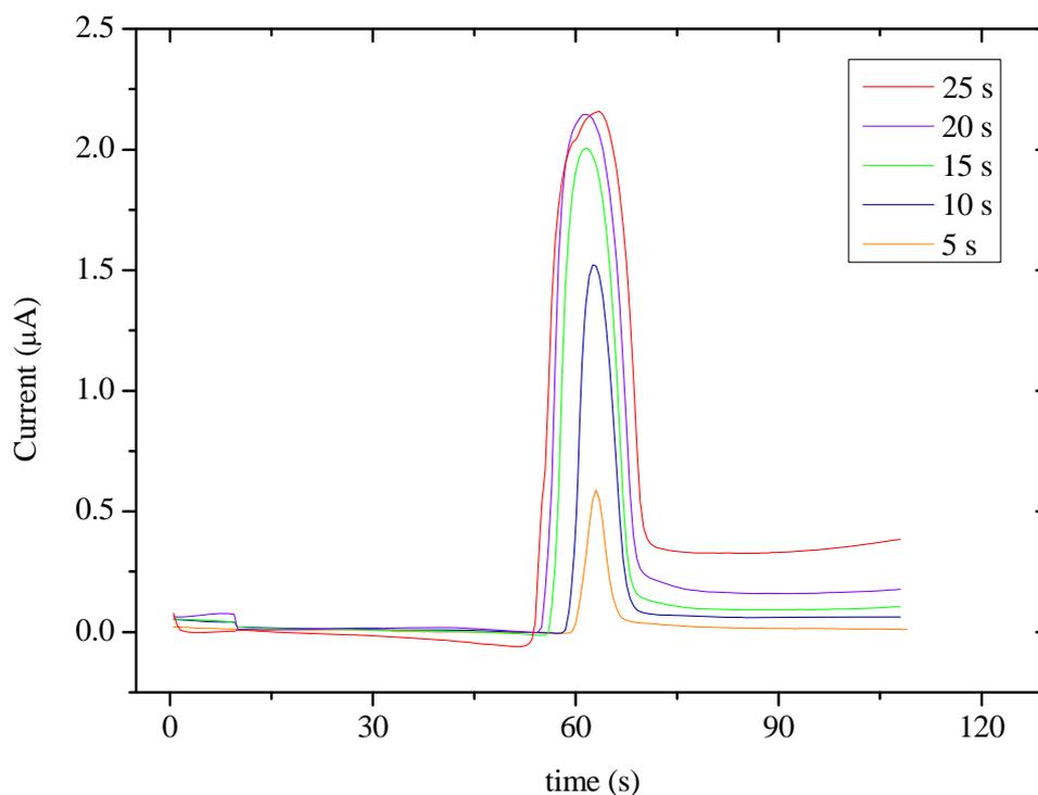
**Figure 4.10** The effect of injection time for PDMS Microchip capillary electrophoresis. The electropherogram of 1 mM of cholesterol at different the injection time, (a) 5 s, (b) 10 s, (c) 15 s, (d) 20 s, and (e) 25 s. Conditions: running buffer, a PB buffer (pH 7.0) solution containing  $0.68 \text{ U}\cdot\text{mL}^{-1}$ ; detection potential, +0.5 V, separation potential, +1600 V; injection potential, +450 V; at  $25 \text{ }\mu\text{m}$  Au wire working electrode.
