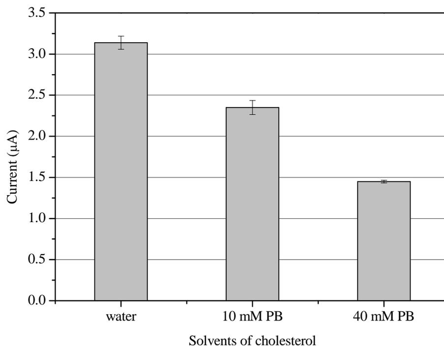
**Figure 4.6** The effect of solvent on peak current of 1 mM Cholesterol. Conditions: running buffer, a PB buffer (40 mM, pH 7.0) solution containing 0.034 U·mL<sup>-1</sup>; detection potential, +0.5 V, separation potential, +1300 V; injection potential, +450 V; injection time, 20 s; at 25 µm Au wire working electrode.
