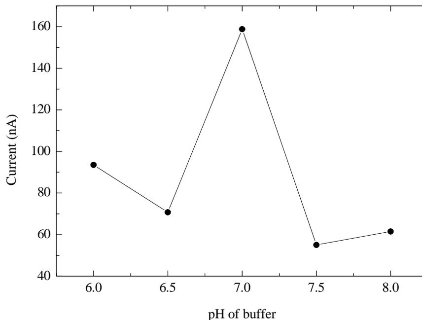
**Figure 4.5** The effect of running buffer pH on peak current of 0.1 mM Cholesterol. Conditions: running buffer, a PB buffer (40 mM, pH 7.0) solution containing  $0.034 \text{ U}\cdot\text{mL}^{-1}$ ; detection potential, +0.5 V, separation potential, +1300 V; injection potential, +450 V; time, 20 s; at  $25 \mu\text{m}$  Au wire working electrode.
