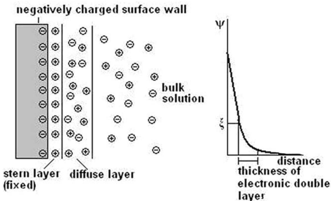
**Figure 2.3** The electric double layers formed next the negative charged solid surface.
