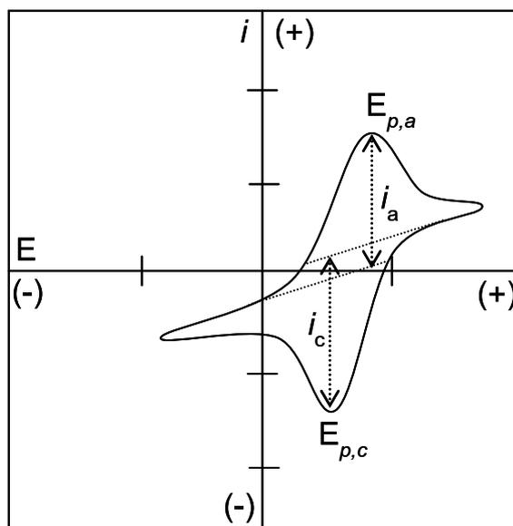
**Figure 2.10** Typical reversible cyclic voltammetry with the initial sweep direction towards more positive potential.
