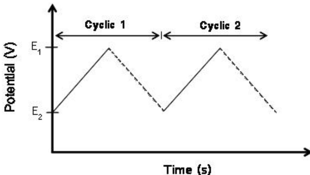
**Figure 2.9** Potential-time profiles used for cyclic voltammetry. Solid line represents forward scan and dashed line represents backward scan.
