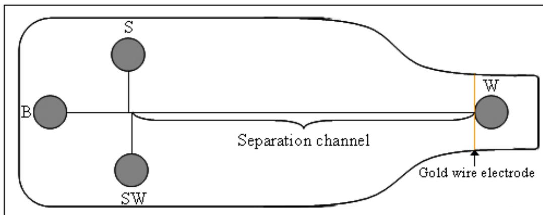
**Figure 3.1** Schematic of PDMS microfluidic device. Channels: 50  $\mu\text{m}$  width, 50  $\mu\text{m}$  depth. 50 mm length of separation channel and 25  $\mu\text{m}$  Au wire working electrode (B = PB buffer + ChOx, S = sample, SW = sample waste, and W = PB buffer).
