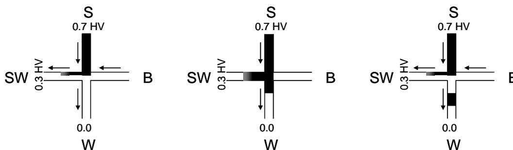
**Figure 2.13** Principle of gated injection. Black stream is the sample, and white stream is the mobile phase. S: sample, SW: sample waste, B: buffer, and W: waste.
