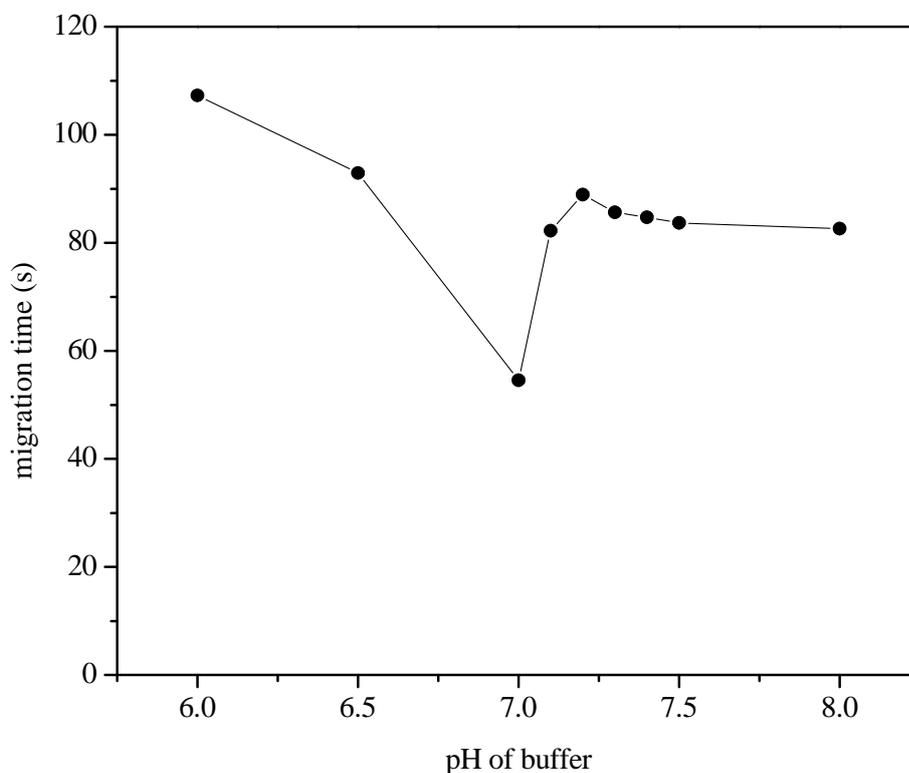
**Figure 4.4** The effect of running buffer pH on migration time of 0.1 mM Cholesterol. Conditions: running buffer, a PB buffer (40 mM, pH 7.0) solution containing 0.034 U·mL<sup>-1</sup>; detection potential, +0.5 V, separation potential, +1300 V; injection potential, +450 V; injection time, 20 s; at 25 μm Au wire working electrode.
