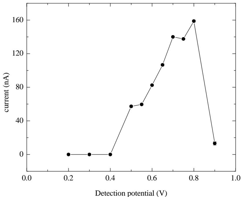
**Figure 4.2** Hydrodynamic voltammogram of 1.0 mM hydrogen peroxide. Conditions: running buffer, a PB buffer (10 mM, pH 7.0) solution; separation potential, +1300 V; injection potential, +450 V; injection time, 20 s; at 25  $\mu\text{m}$  Au wire working electrode.
