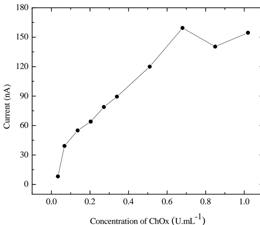
**Figure 4.7** The effect of the enzyme cholesterol oxidase containing in PB buffer (40 mM, pH 7.0) on peak current of 1 mM Cholesterol. Conditions: detection potential, +0.5 V, separation potential, +1300 V; injection potential, +450 V; inject time, 20 s; at 25  $\mu\text{m}$  Au wire working electrode.
