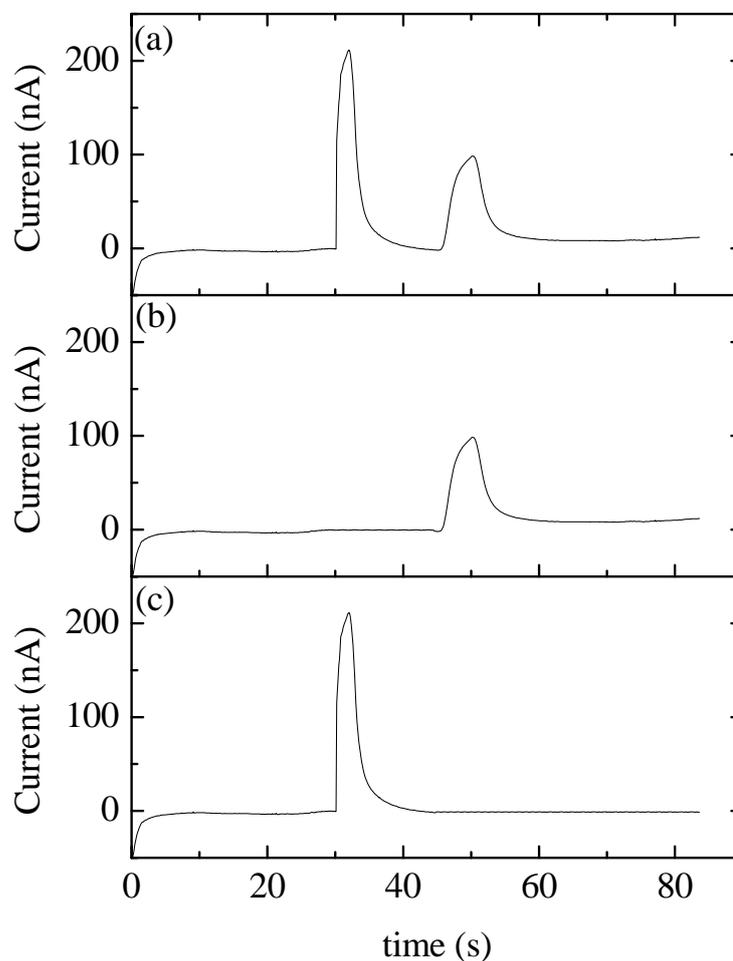
**Figure 4.1** The characterization of PDMS Microchip capillary electrophoresis (a) Electrochromatogram of mixed 250  $\mu\text{M}$  dopamine and 250  $\mu\text{M}$  catechol, (b) and (c) is 250  $\mu\text{M}$  dopamine and 250  $\mu\text{M}$  catechol, respectively. Conditions: running buffer, a MES buffer (20 mM, pH 7.0) solution; separation potential, +1300 V; injection potential, +450 V; injection time, 20 s; detection potential, +0.8 V at 25  $\mu\text{m}$  Au wire working electrode.
