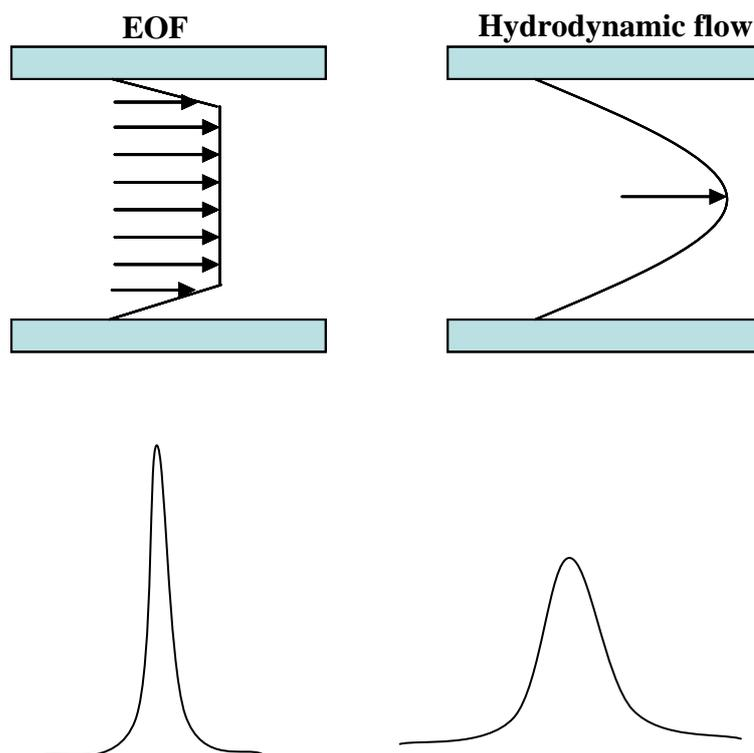
**Figure 2.5** Flow profile and effect on peak shapes for electroosmotic flow and laminar flow.
