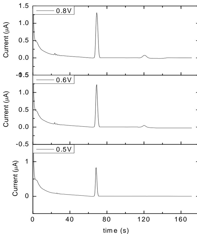
**Figure 4.12** The effect of interference for PDMS Microchip capillary electrophoresis. The electrochromatogram of 1 mM of cholesterol and 0.5 mM ascorbic acid at different the detection potential, (a) +0.5 V, (b) +0.6 V, and (d) +0.8 V. Conditions: running buffer, a PB buffer (pH 7.0) solution containing  $0.68 \text{ U}\cdot\text{mL}^{-1}$ , separation potential, +1600 V; injection potential, +450 V; time, 20 s; at  $25 \text{ }\mu\text{m}$  Au wire working electrode.
