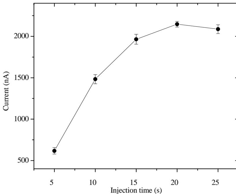
**Figure 4.11** The effect of injection time on the migration time of 0.1 mM Cholesterol. Conditions: running buffer, a PB buffer (40 mM, pH 7.0) solution containing 0.68  $\text{U}\cdot\text{mL}^{-1}$ ; detection potential, +0.5 V, separation potential, +1600 V; injection potential, +450 V; at 25  $\mu\text{m}$  Au wire working electrode.
