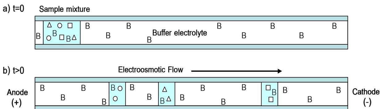
**Figure 2.6** Separation mechanism in CZE, where B represents buffer, a) Sample mixture is introduced into capillary; b) voltage is applied, and the analytes separate into distinct zones.
