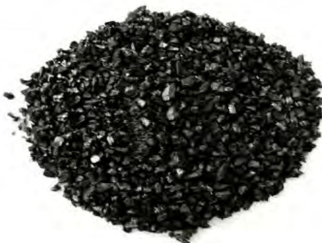
Figure 2.2 Granular activated carbon.
