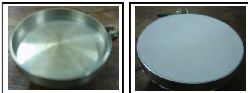
Figure 3.5: The photograph of circular holder for holding cotton sample fabrics.
