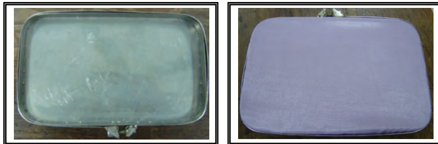
Figure 3.6: The photograph of rectangular holder for holding PET sample fabrics.
