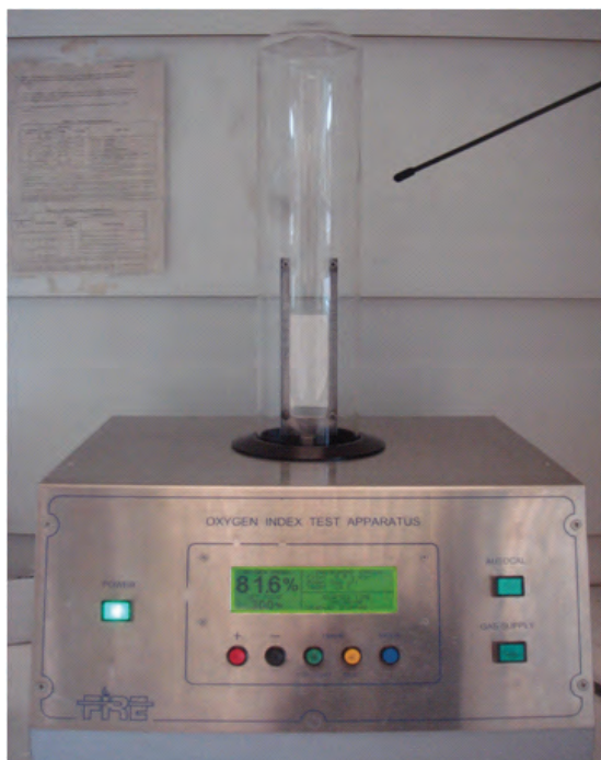
Figure 3.20: Photograph of the Limiting Oxygen Index (LOI) test
