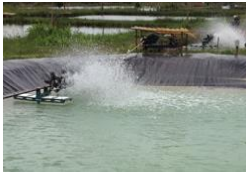
(c) Mechanical surface aerator or paddle wheels
