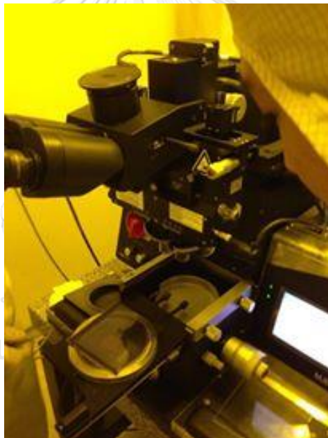
Figure 4.7: UV light through the mask onto the coated wafer.
