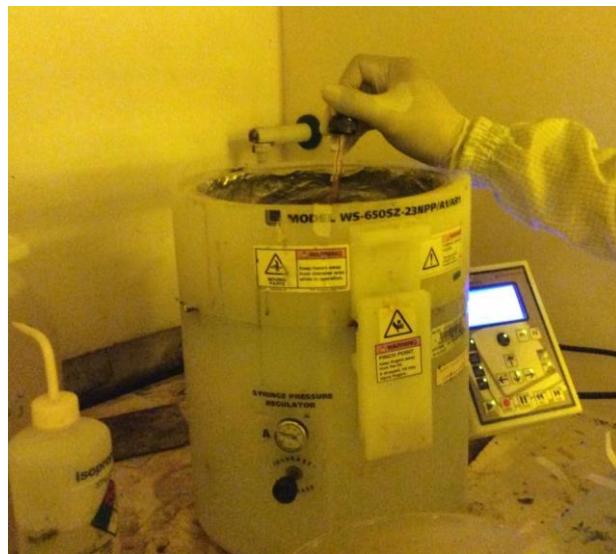
Figure 4.5: Spin coating the substrate with the photoresist.
