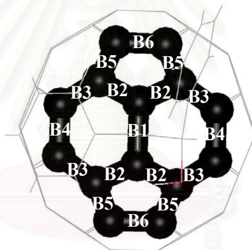
Figure 4.5 The six selected bond lengths on the C_{60} surface which are in the region 5 Å from the bridged atoms.
