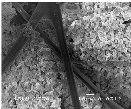
Figure 4.14 TSSC inner surface at the end of the continuous fermentation (16 days)
