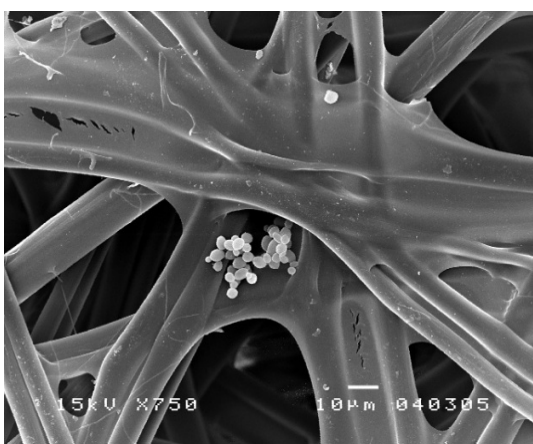
Figure 4.12 TSSC outer surface at the end of the continuous fermentation (16 days)
