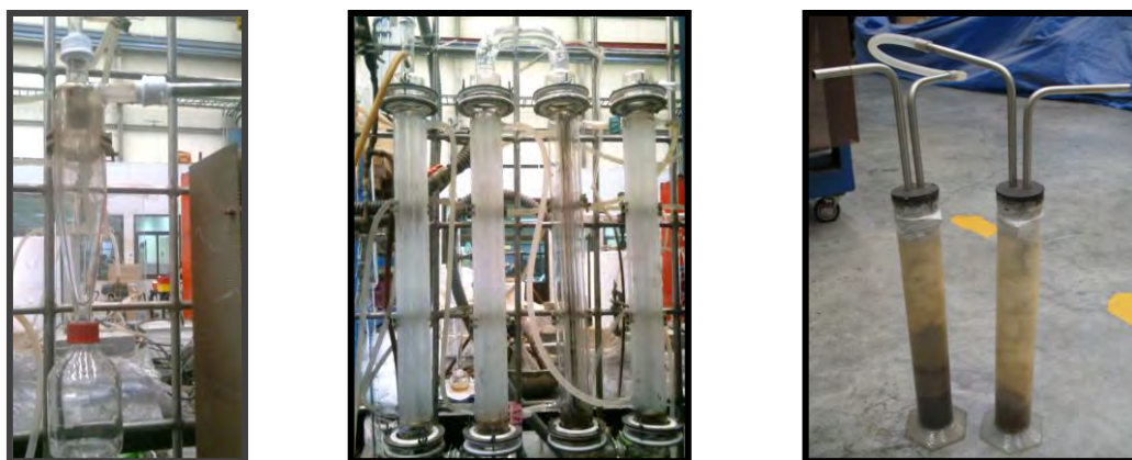
Figure 3.14 Cyclone, Condensers and Washer (from right to left)
