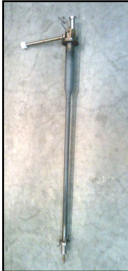
Figure 3.10 Tubular Stainless Steel Reactor
