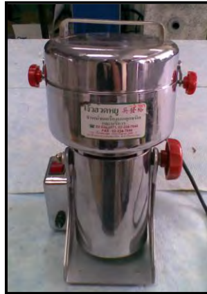
Figure 3.5 High Speed Crusher Machine
