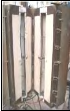
Figure 3.11 Vertical tubular furnace
