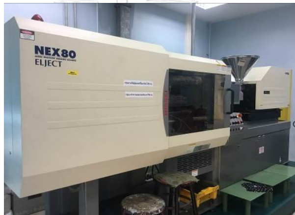
Figure 3.13 Injection molding machine (NEX80 Nissei, USA)
