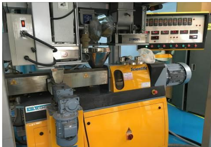
Figure 3.6 Twin Screw Extruder (LTE26-40 Labtech Scientific)
