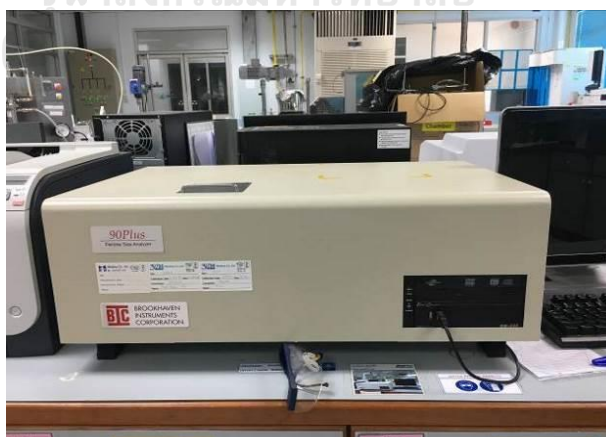
Figure 3.7 Particle size analyzer (90Plus, Brookhaven USA)
