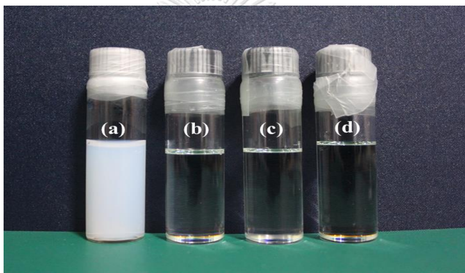
Figure 4.4 A 12 wt% Silica dispersion (in water) and 12 wt% HDTMS-silica dispersion (in toluene) b HDTMS-silica1, c HDTMS-silica2, and d HDTMS-silica3
