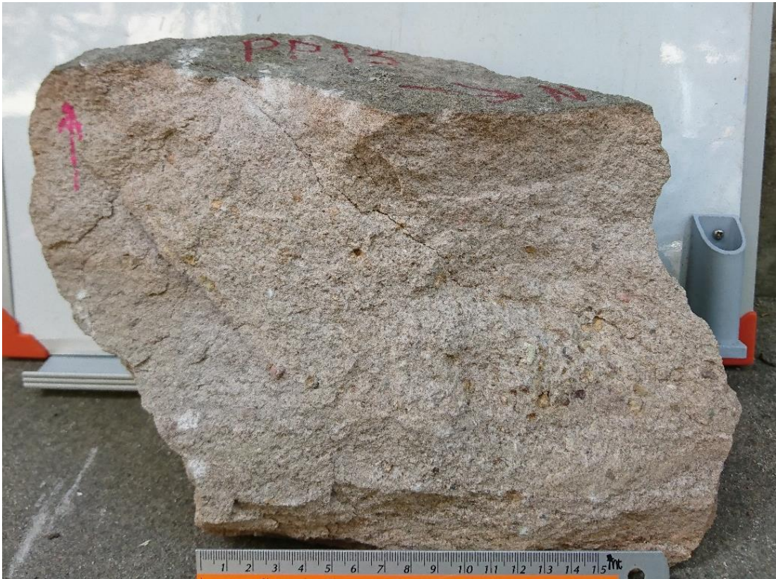
Figure 48 White, medium-grained sandstone of the Phu Phan Formation (sample no. PP14).
