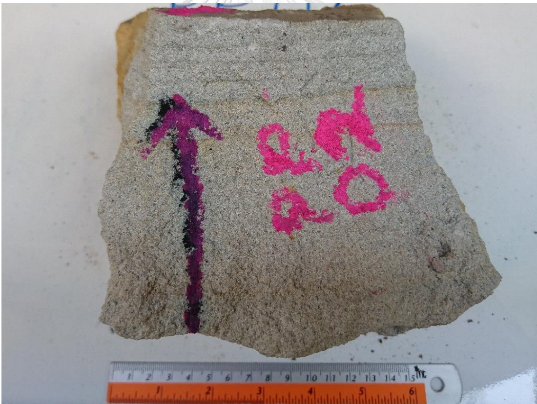
Figure 4.25 A hand specimen of Whitish grey, medium-grained sandstone with well lamination of the Phra Wihan Formation (sample no. PP02).
