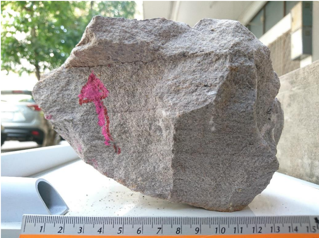
Figure 51 White, medium-grained sandstone of the Phu Phan Formation (sample no. PP15).
