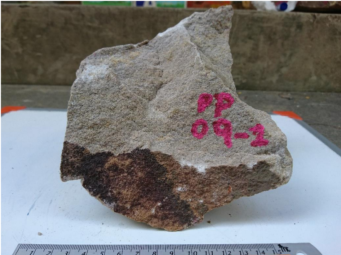
Figure 33 Whitish grey, medium grained sandstone of the Phra Wihan Formation (sample no. PP09).
