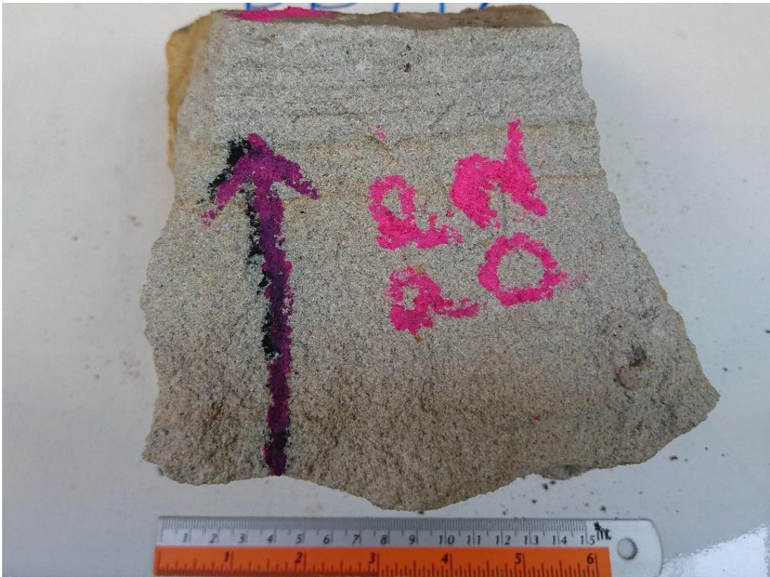
Figure 5 Whitish grey, medium-grained sandstone with well lamination of the Phra Wihan Formation (sample no. PP02).
