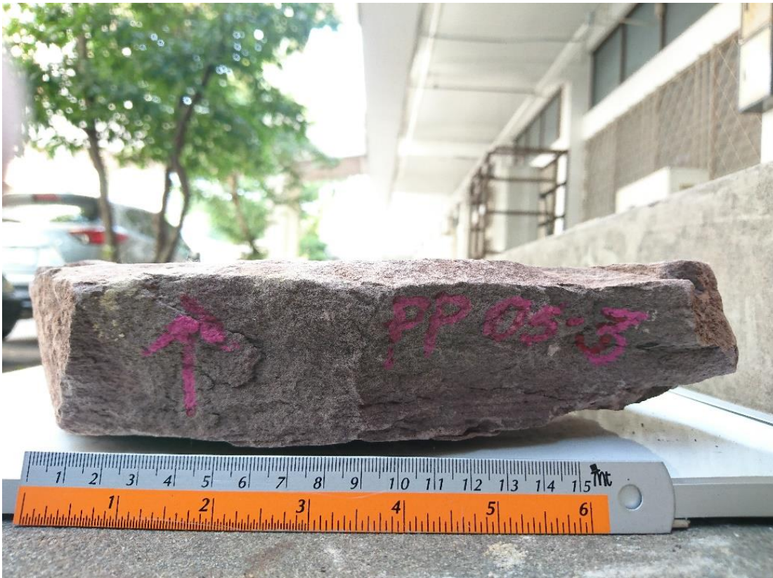
Figure 4.28 A handspecimen of Reddish grey, fine-grained sandstone with faint lamination of the Sao Khua Formation (sample no. PP05-3),
