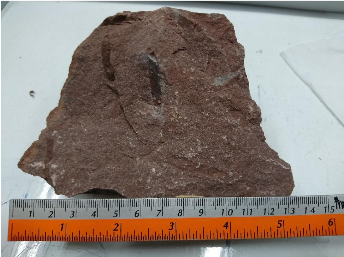
Figure 60 Reddish brown fine-grained sandstone of the Phu Phan Formation (sample no. PTT15).
