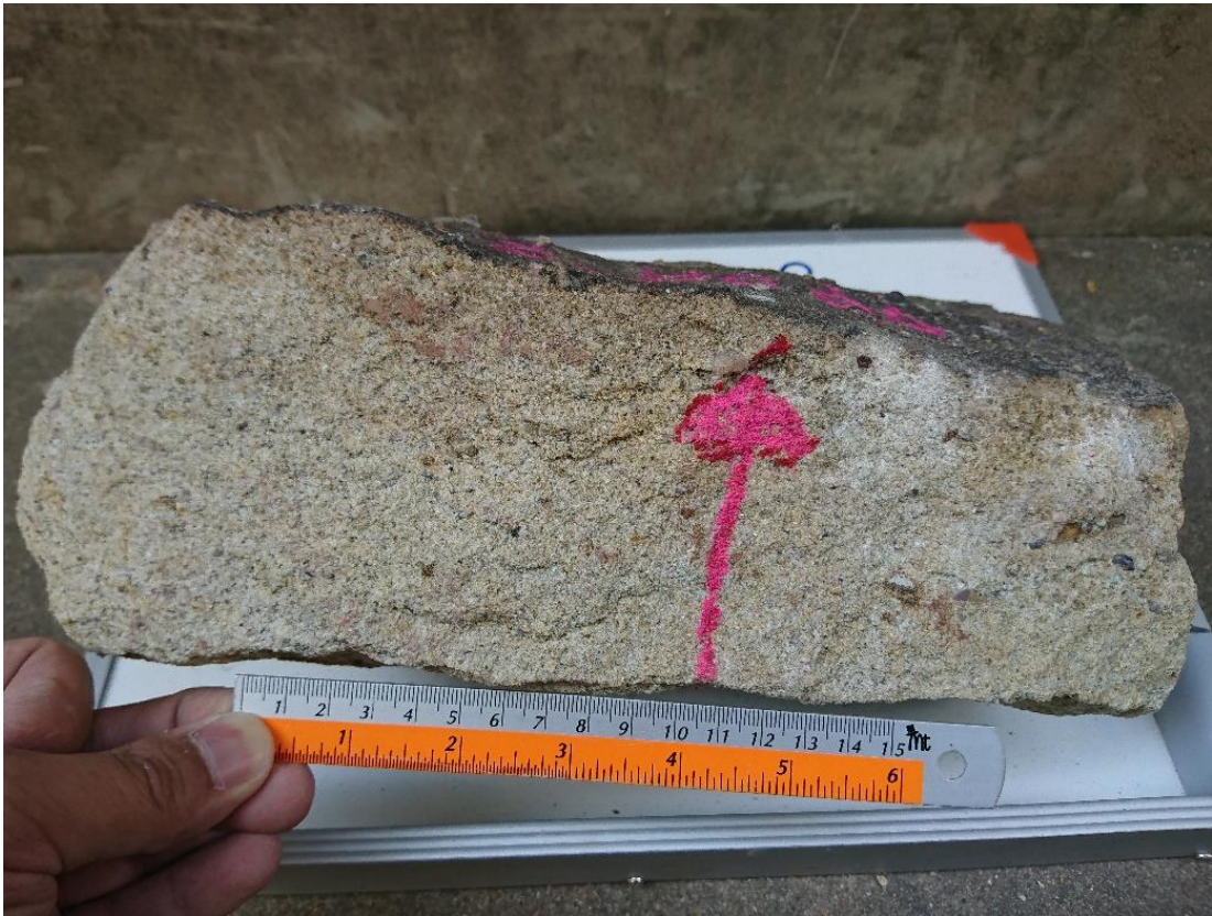
Figure 14 Whitish grey, medium-grained sandstone of the Phu Phan Formation (sample no. PP04-2).
