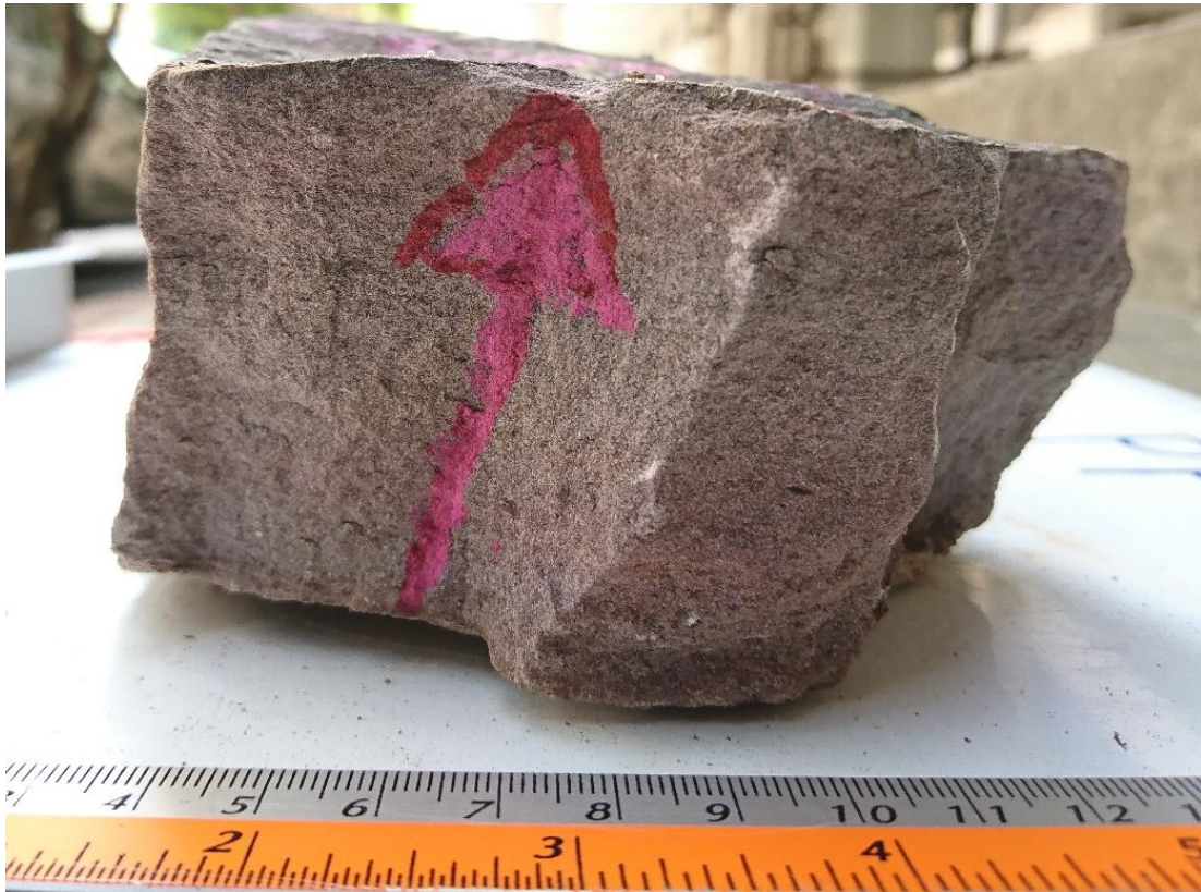
Figure 19 Reddish grey, fine-grained sandstone with faint lamination of the Sao Khua Formation (sample no. PP05-2).
