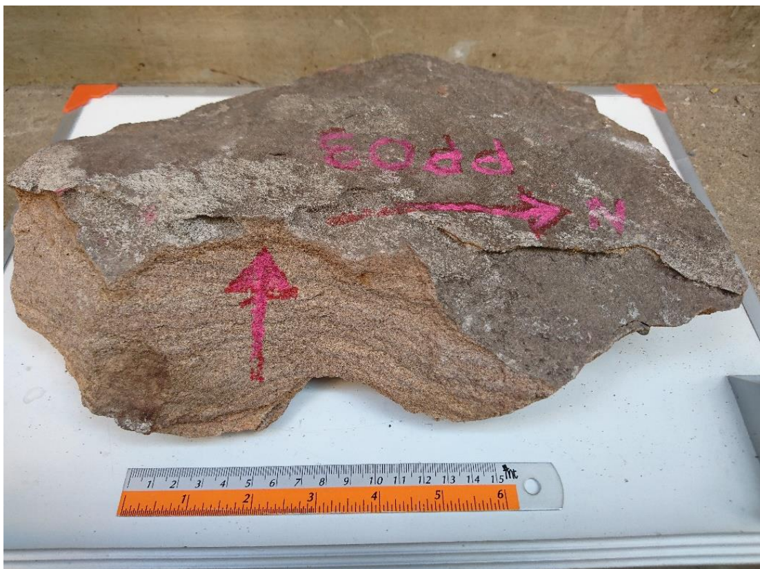
Figure 8 Reddish-brown, medium-grained sandstone with well lamination of the Sao Khua Formation (sample no. PP03).
