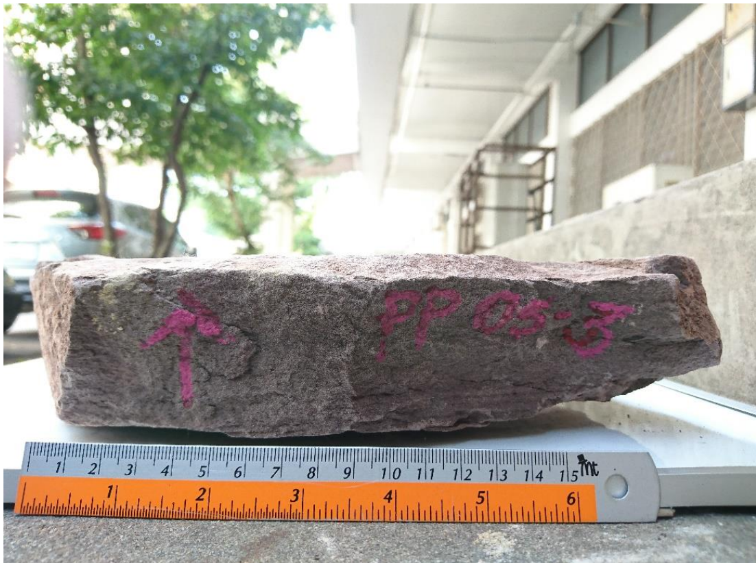
Figure 21 Reddish grey, fine-grained sandstone with faint lamination of the Sao Khua Formation (sample no. PP05-3),
