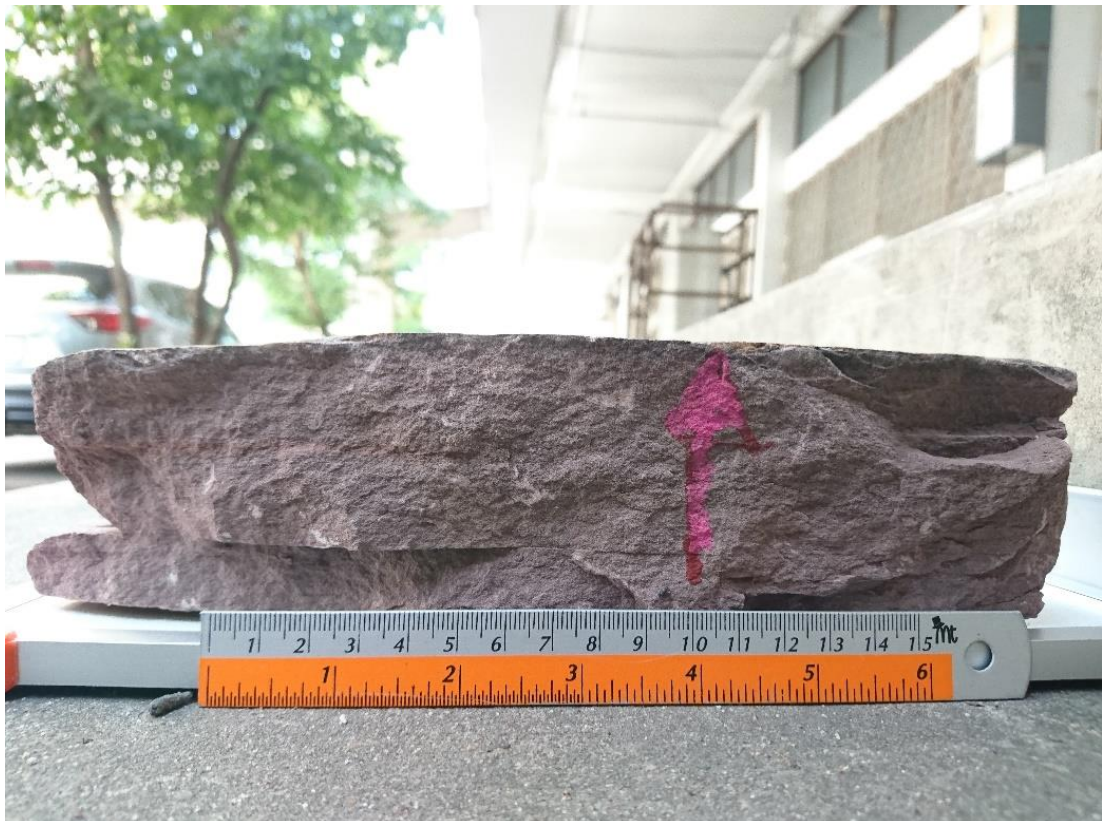
Figure 24 Reddish grey, fine-grained sandstone with faint lamination of the Sao Khua Formation (sample no. PP06).
