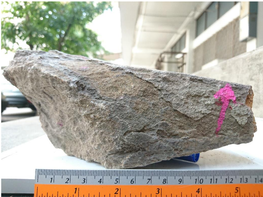
Figure 27 Whitish orange, medium grained sandstone of the Phu Phan Formation (sample no. PP07).
