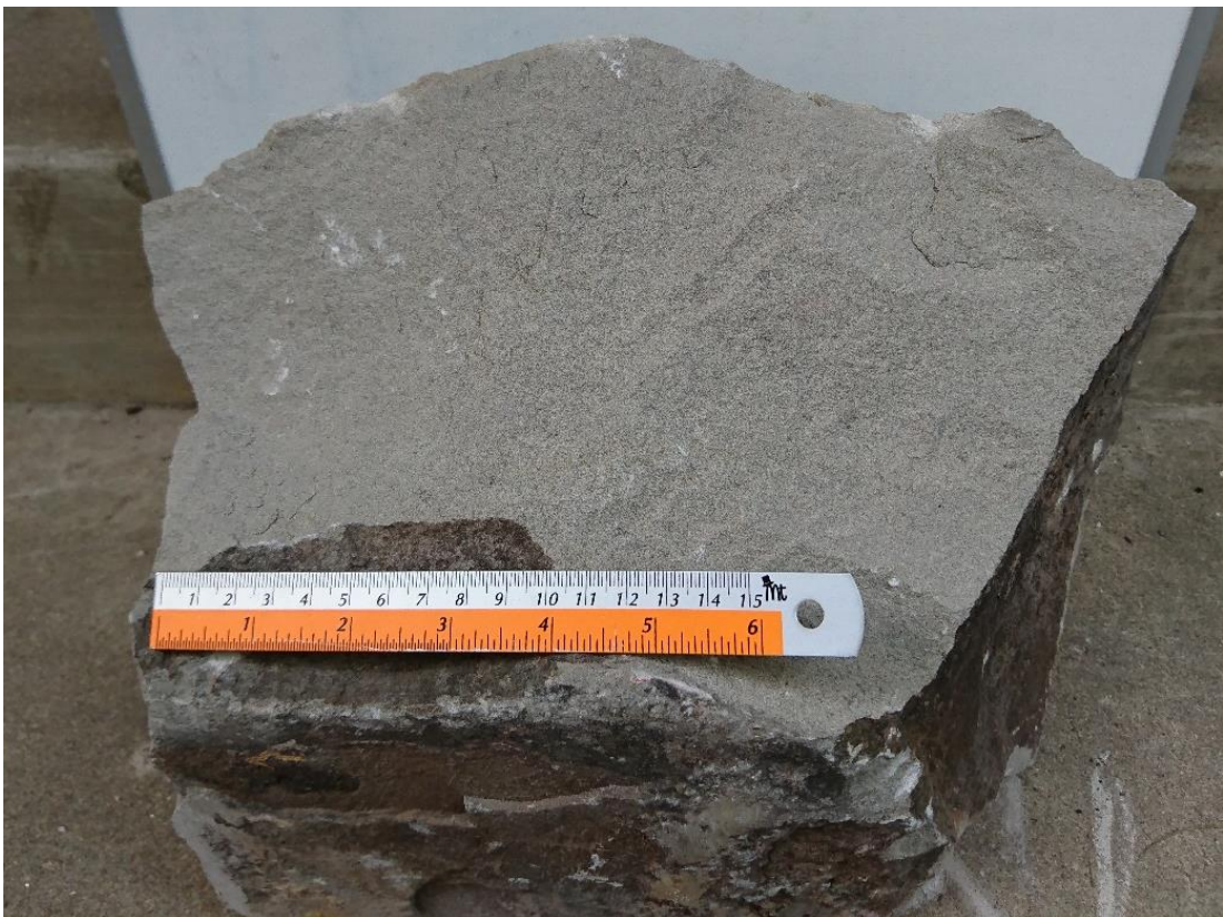
Figure 2 Greenish-gray very fine-grained sandstone of the Phu Kradung Formation sample no. PP01.
