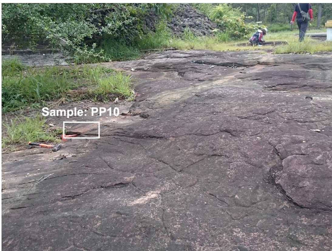
Figure 35 Natural outcrop of sandstone of the Phu Phan Formation at Wat Tham Pha Mong, Mueang Mukdahan District, Mukdahan Province (Orange sledge hammer, 32.5 cm-long, is to scale). White rectangle is the sampling site.
