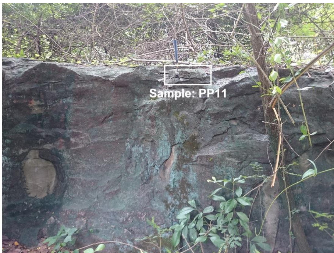
Figure 38 Natural outcrop of sandstone of the Sao Khua Formation in front of Wat Phuttha Kiri, Nong Sung District, Mukdahan Province (Geological hammer, 32.5 cm-long, is to scale). White rectangle is the sampling site.
