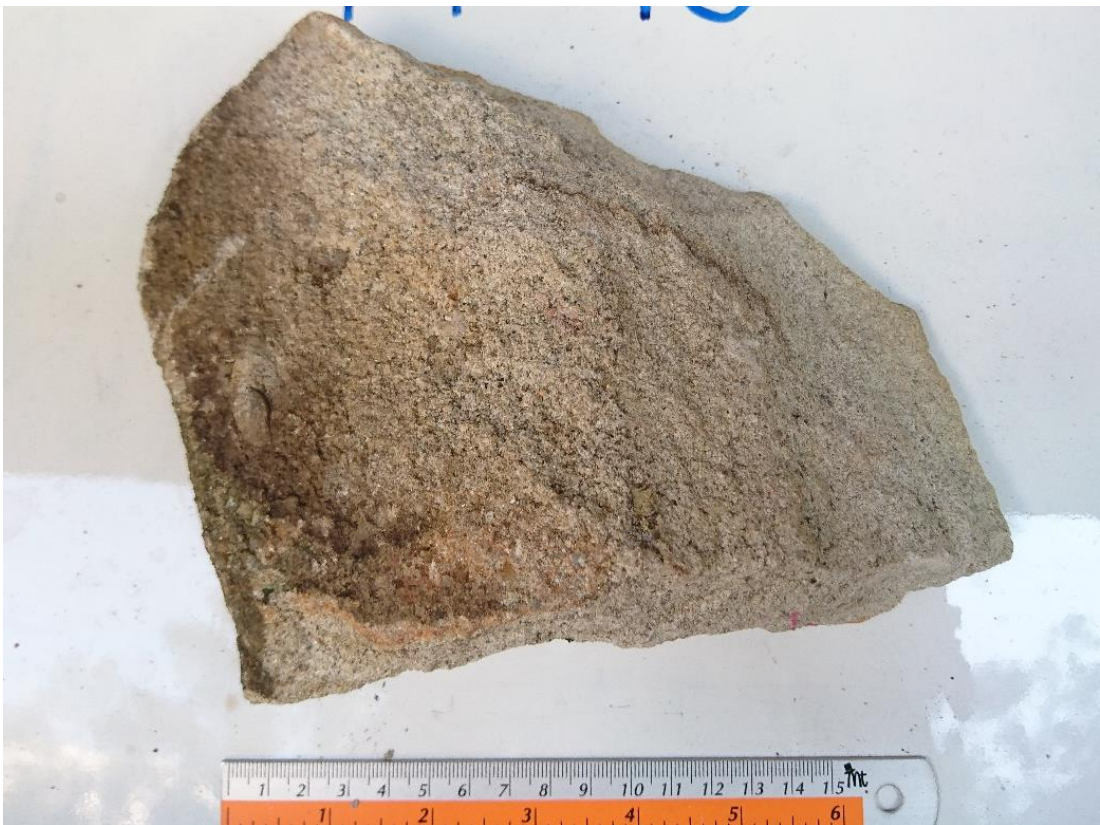
Figure 36 Brownish white, medium-grained sandstone of the Phu Phan Formation (sample no. PP10).
