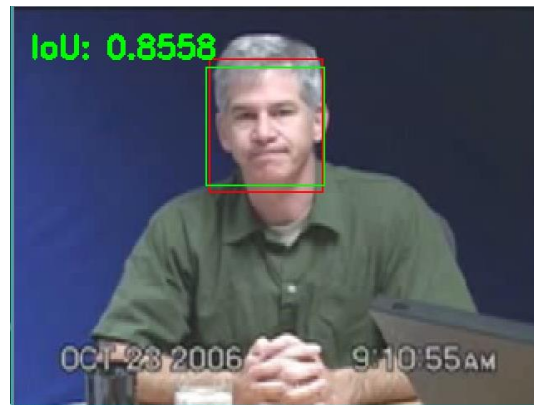
Figure 4.7. Example of IOU in face detection. Green bounding box is a GT and red bounding box is SUT.
