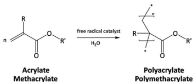
Figure 2.5 The synthesis route of polyacrylate or polymethacrylate with the acrylate linkage -(\text{C}=\text{O})-\text{O}- .
