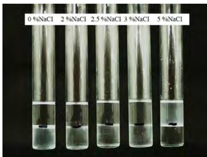
Figure C15 Salinity scan for 0.1 M C12-14EO5 with Hexadecane at 95 °C.
