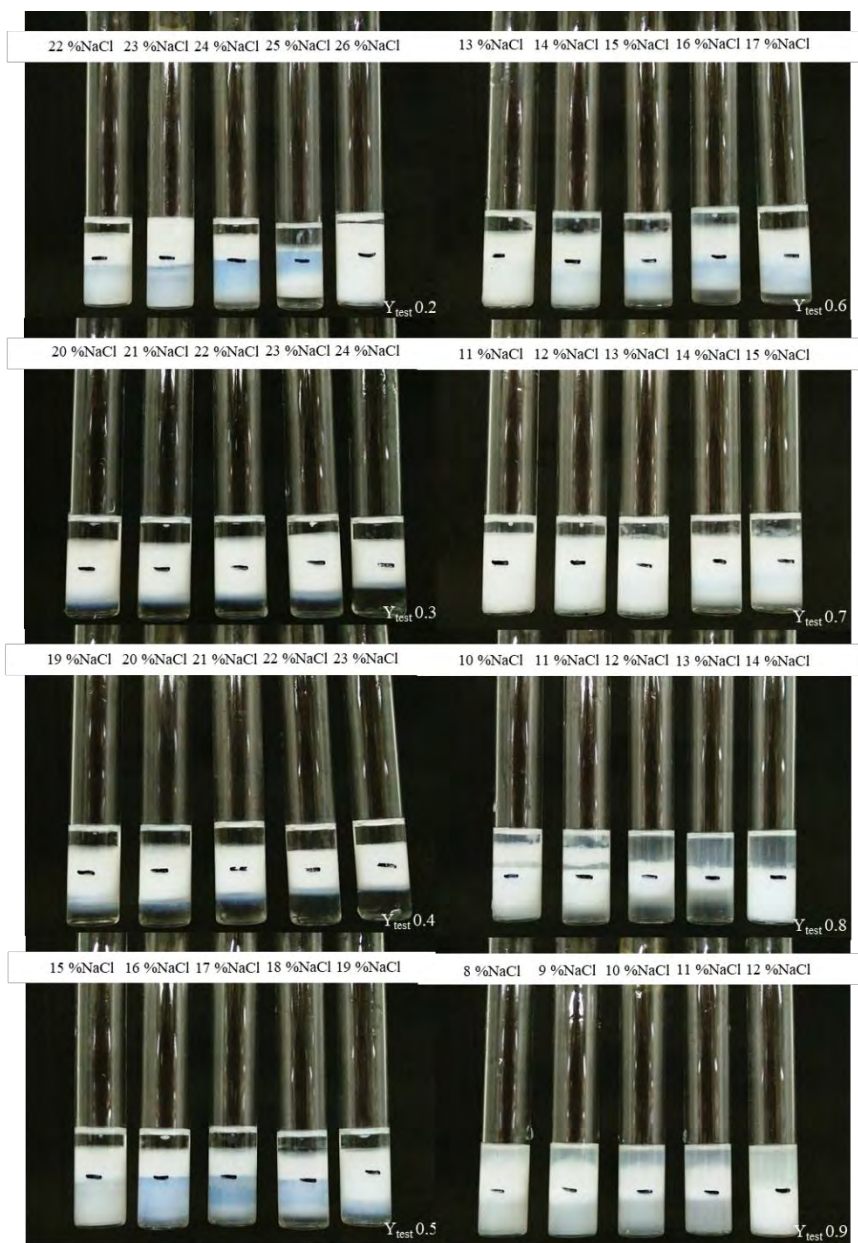
Figure E42 Salinity scan of mixed C12-14EO9 and C16-18PO2EO4 with Decalin.
