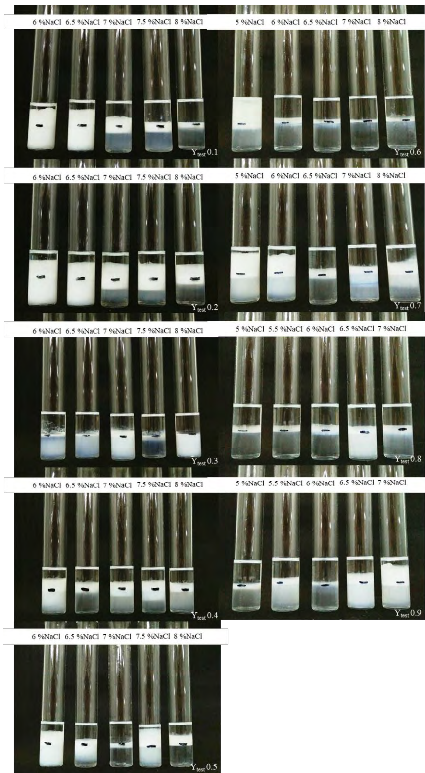
Figure E4 Salinity scan of mixed C12-14EO3 and C12-14EO2 with Cyclohexane.
