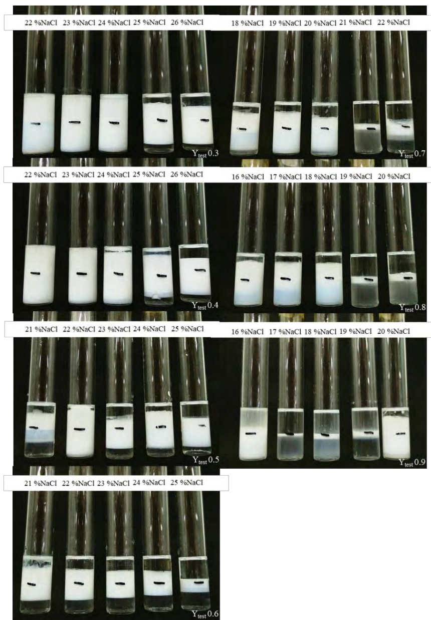
Figure E36 Salinity scan of mixed C12-14EO9 and C12-14EO2 with Decalin.
