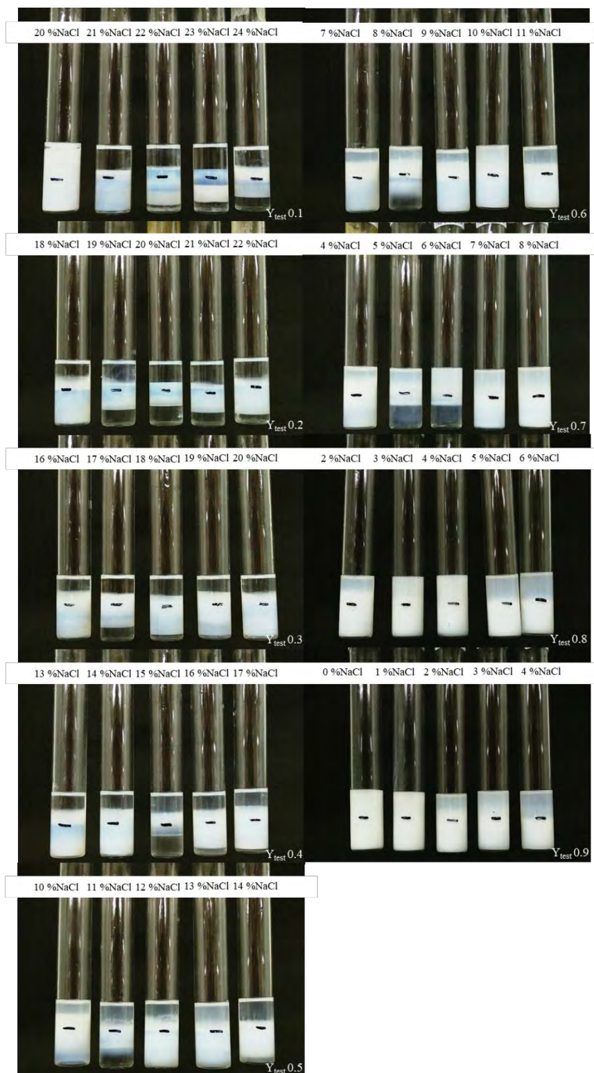
Figure E43 Salinity scan of mixed C12-14EO9 and C16-18PO4EO6 with Cyclohexane.
