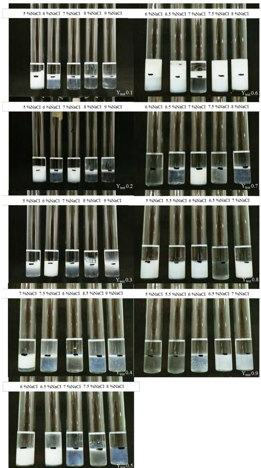
Figure E3 Salinity scan of mixed C12-14EO3 and C12-14EO1 with Decalin.
