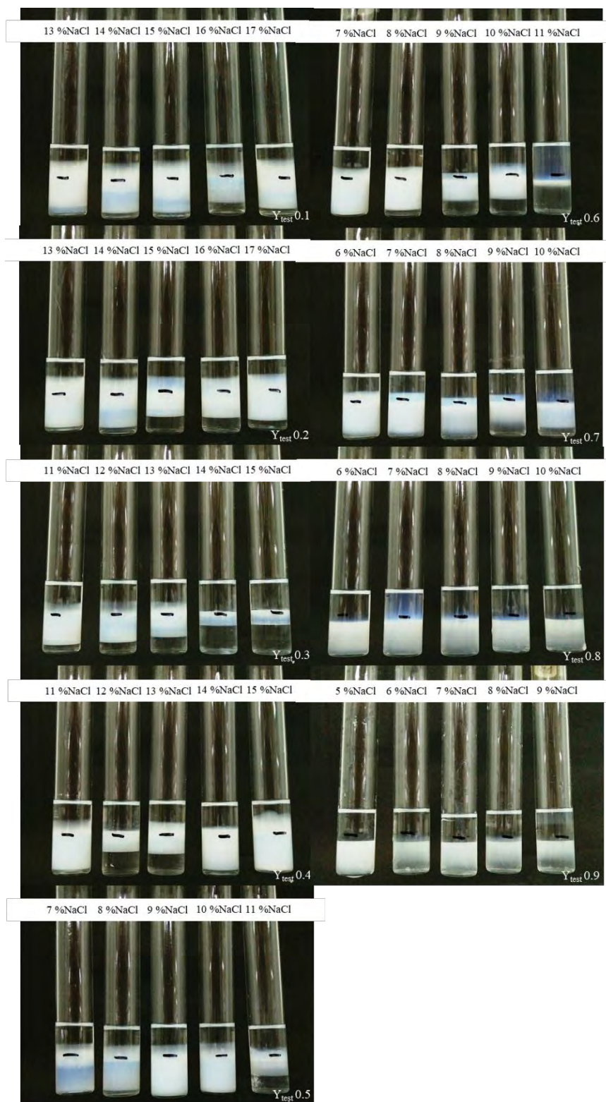
Figure E26 Salinity scan of mixed C12-14EO5 and C16-18PO2EO4 with Heptane.
