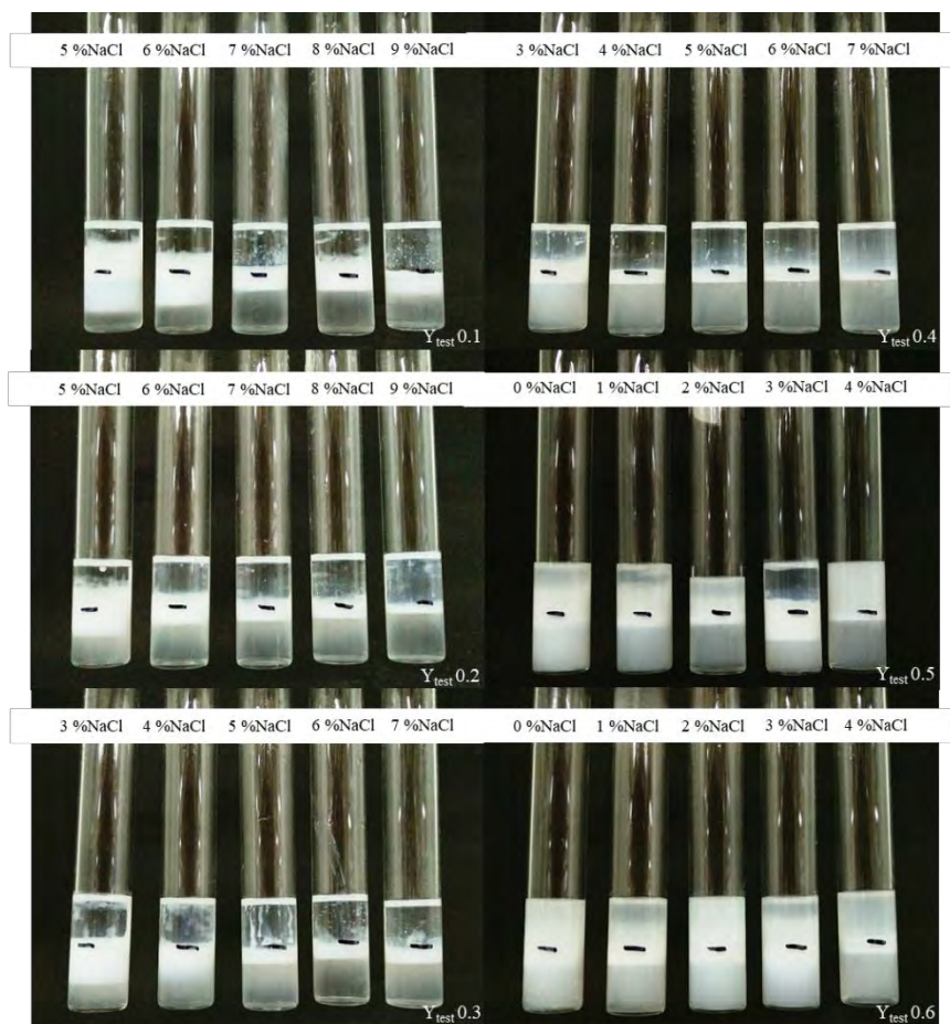
Figure E12 Salinity scan of mixed C12-14EO3 and C16-18PO2EO4 with Decalin.
