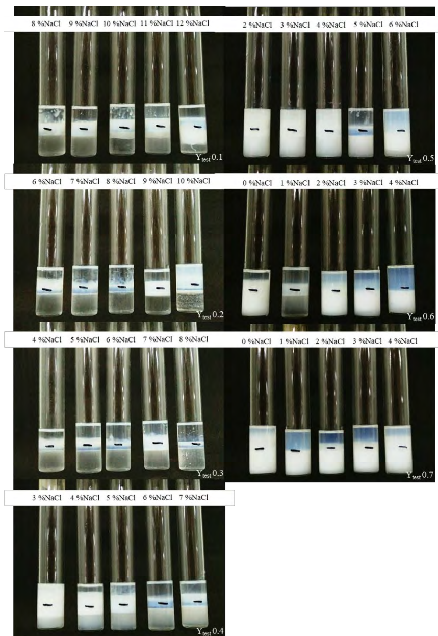
Figure E28 Salinity scan of mixed C12-14EO5 and C16-18PO4EO6 with Cyclohexane.
