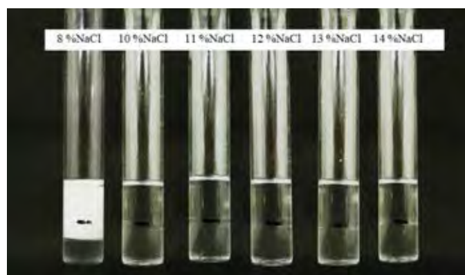
Figure D10 Salinity scan for 0.1 M C12-14EO9 with Hexadecane at 75 °C.
