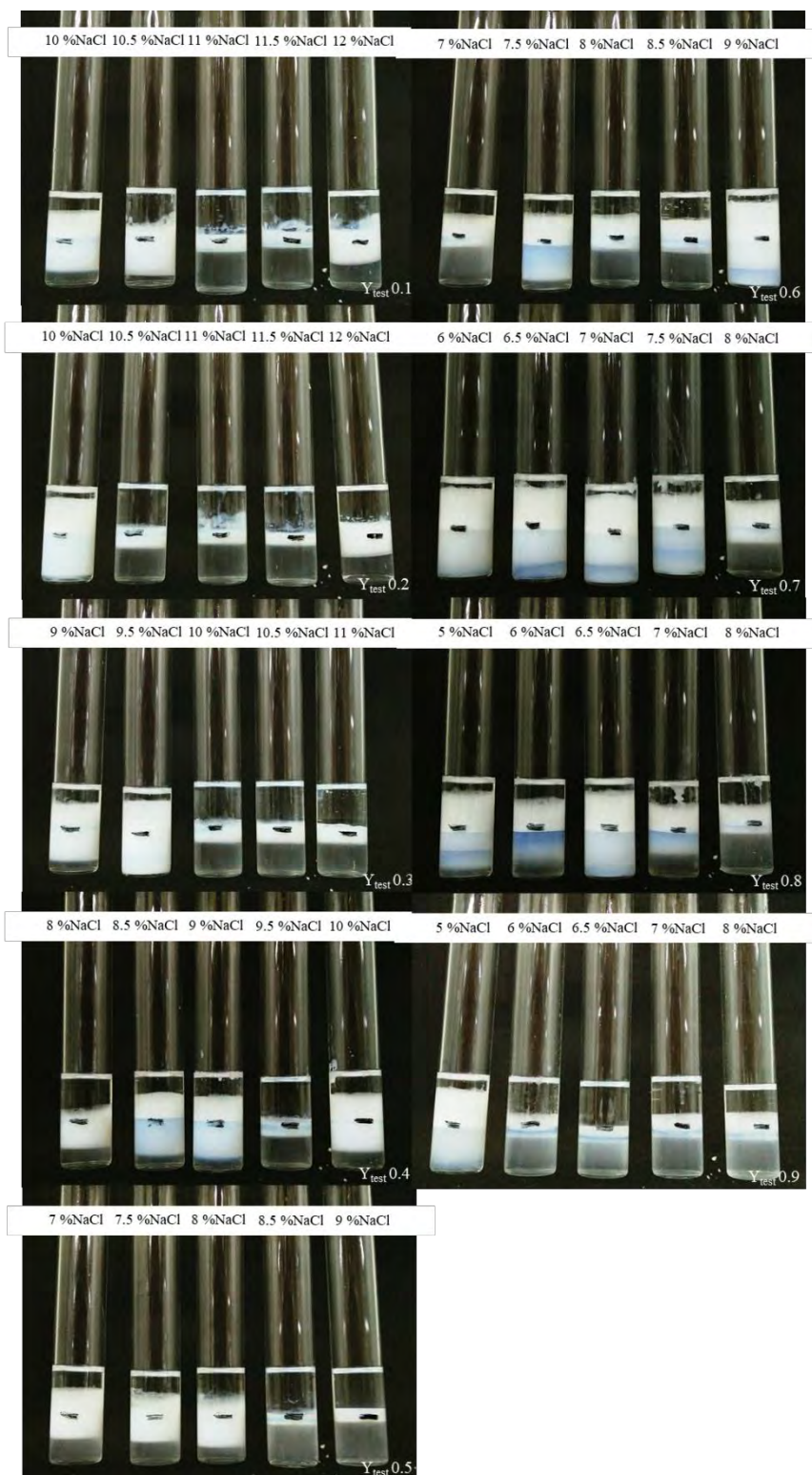
Figure E19 Salinity scan of mixed C12-14EO5 and C12-14EO2 with Cyclohexane.
