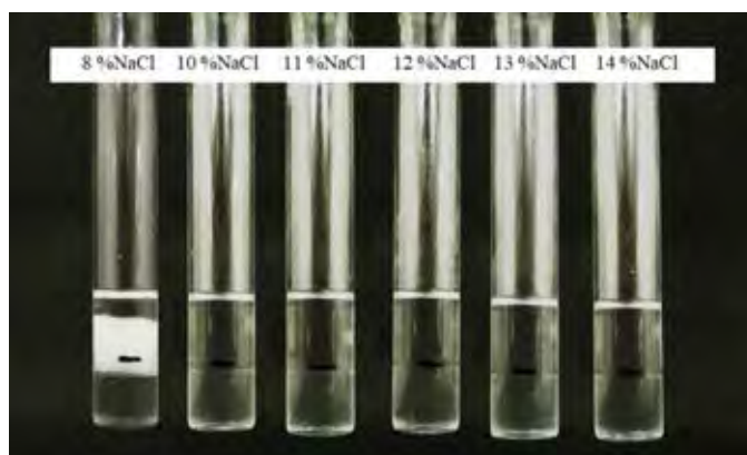
Figure D11 Salinity scan for 0.1 M C12-14EO9 with Hexadecane at 80 °C.
