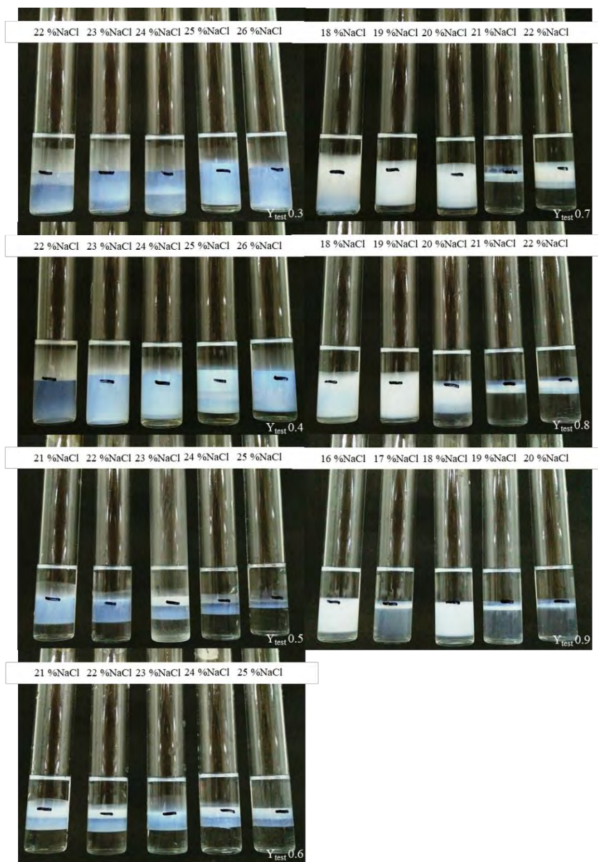
Figure E35 Salinity scan of mixed C12-14EO9 and C12-14EO2 with Heptane.
