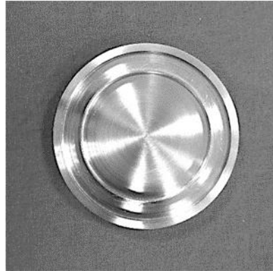
Figure 5 A stainless steel mould (a diameter of 50 \pm 1 mm and a depth of 3.0 \pm 0.1 mm)
