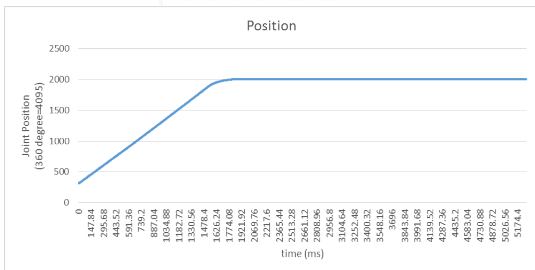
Figure 45: Joint Position When Moving Forward
