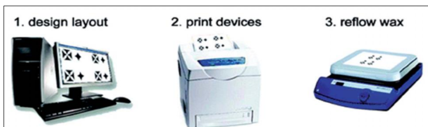
Figure 2.7 Patterning hydrophobic barriers in paper by wax printing. (1) Designed Pattern of PADs using computer software, (2) printing pattern by wax printer and (3) melting wax by hot plate for create hydrophilic channel.
