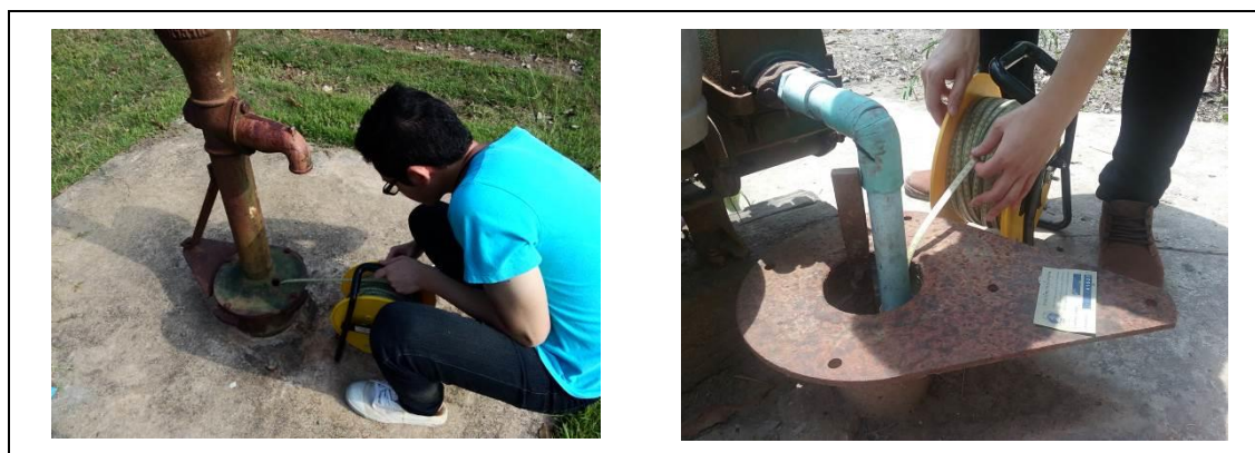
Figure 4. 3 Groundwater data levels collection
