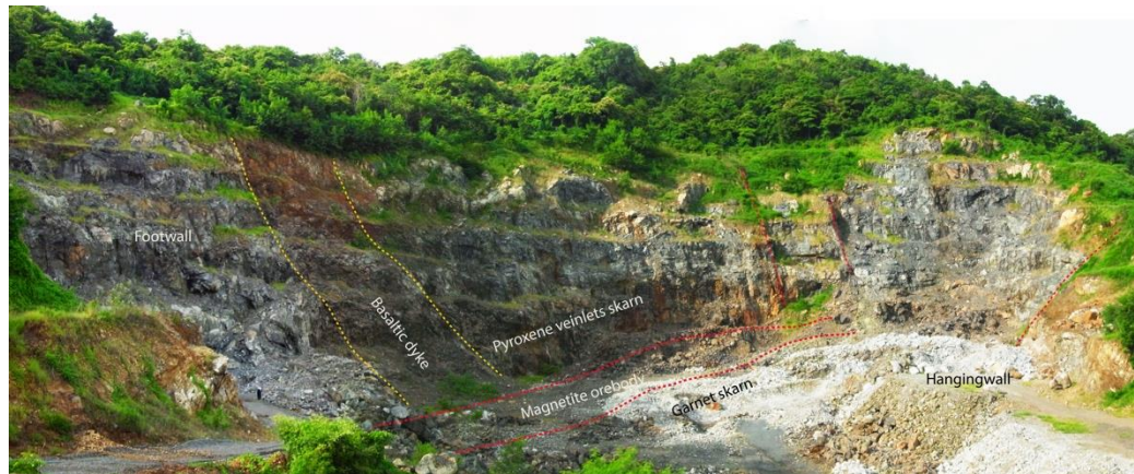
Figure 3. 5. Panorama view of Khao Lek open pit showing volcanics protolith on footwall and the main orebody that is enclosed by garnet skarn zone (white) on pit floor. Photo looking northeast.
