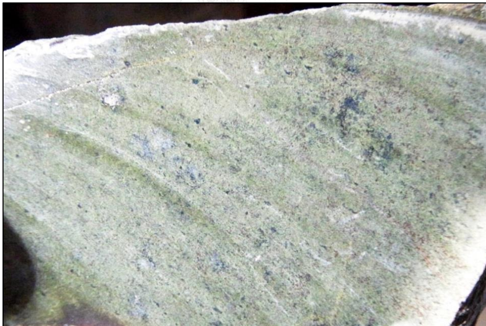
Figure 4. 10 Photograph of dyke skarn showing green pyroxene skarn. Note that some magnetite patches present (top right).
