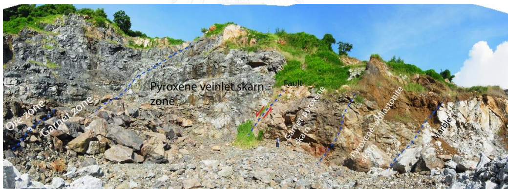
Figure 3. 3 Panorama view of Khao Lek open pit for eastern pit wall showing the end of main orebody (left of photograph), volcanics with pyroxene skarn veinlets, garnet-pyroxene skarn (brown), narrow pyroxene-wollastonite skarn and marble (white, right). Photograph looking northeast.
