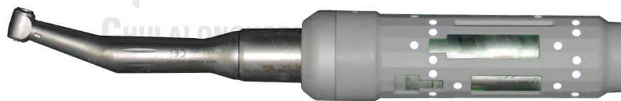
Figure 6. Implant headpiece attached with headpiece tracking sensor
