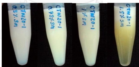
Figure 5 Physical appearances of 0.5 %, 0.75 %, 1 %, 1.5 %w/w silymarin nanoemulsions (F1) after centrifugation from left to right, respectively.
