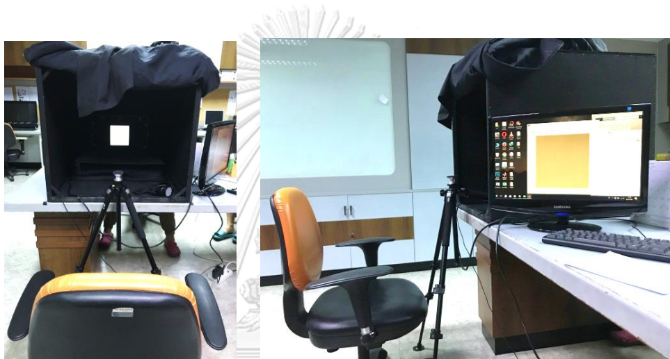
Figure 3.6 Experimental box with black fabric and chin rest stand.
