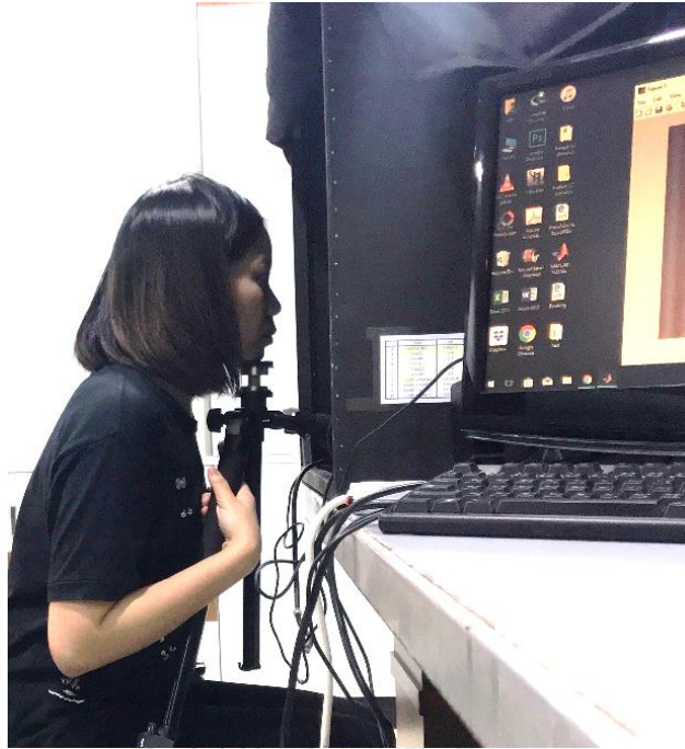
Figure 3.8 Before an observer is covered with black fabric, she/he sat in front of the display and located chin on the chin rest.
