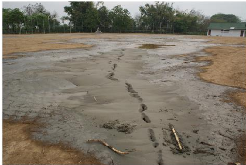
Figure 2.7. A sand boiling phenomenon caused by 24 th March 2011 Earthquake (Ruangrassamee et al., 2012)
