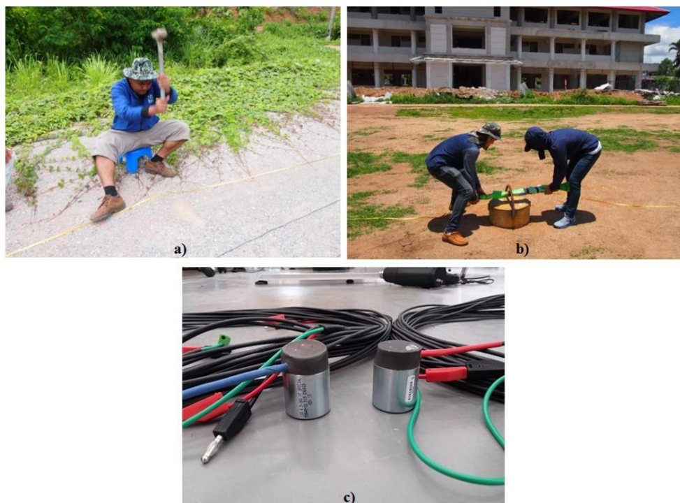
Figure 5.9. Equipment used for SASW measurement (a) a sledge hammer, (b) a drop weight, and (c) two geophone receivers.
