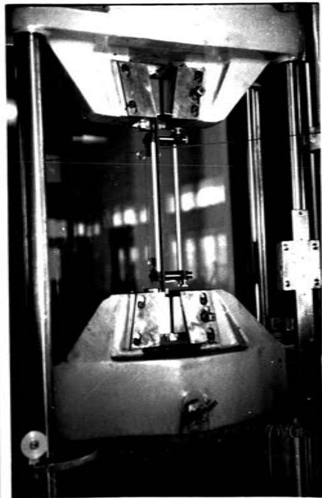
Fig. A7 - Method of testing specimen in tension. The extensometer shown has 8 inches gauge length (magnification 5:1).
