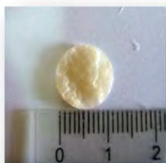
Figure 3.9 The circular piece of freeze dried BC-alginate at the diameter of 1.20 cm and the thickness of 3 mm.
