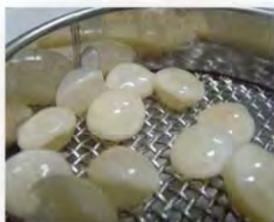
Figure 3.12 Enzyme immobilized by double layers entrapment of calcium alginate with a diameter of 1.60 cm.
