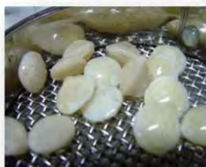
Figure 3.10 Fifteen circular pieces of freeze dried BC-alginate was soaked in 3ml of enzymatic solution for 30 min.
