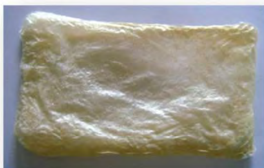
Figure 3.7 Form of the fresh BC-alginate after cross-linked by 0.12 M calcium chloride for 24 h.
