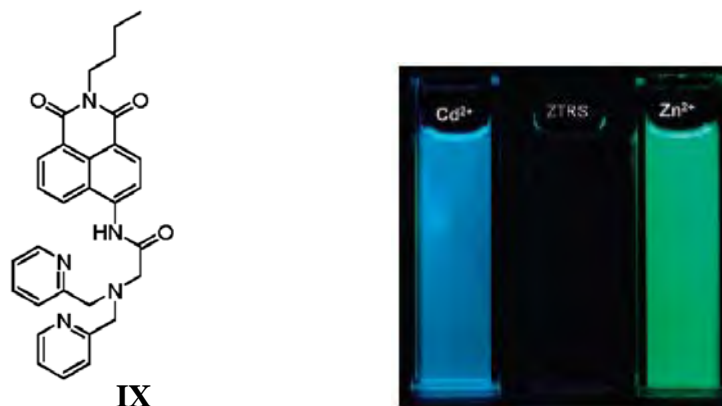
Figure 1.11 The structure of IX and its fluorogenic responses toward \text{Cd}^{2+} and \text{Zn}^{2+}
