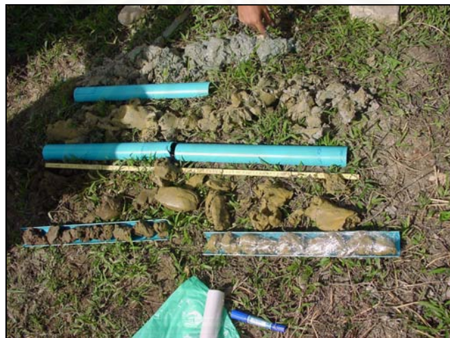
Figure 2.18 Samples from borehole were collected
