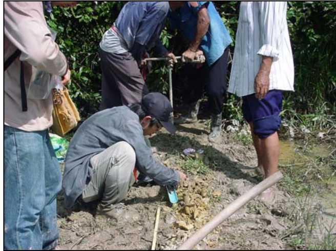
Figure 2.17 Hand auger is the application tool used in the field
