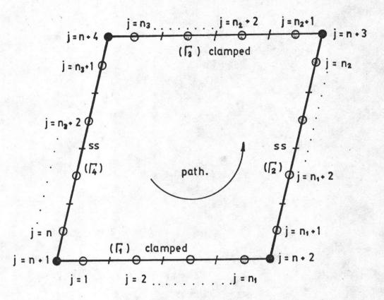
FIG.12 Boundary Discretization
