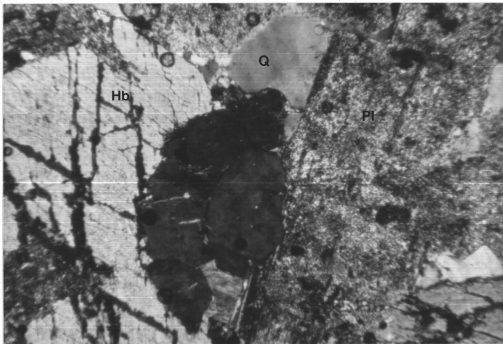
Fig. 3.3 Photomicrograph of diorite in Phai Sali area showing sericitization and saussuritization of plagioclase (Pl) (X-nicols, 45 x).
