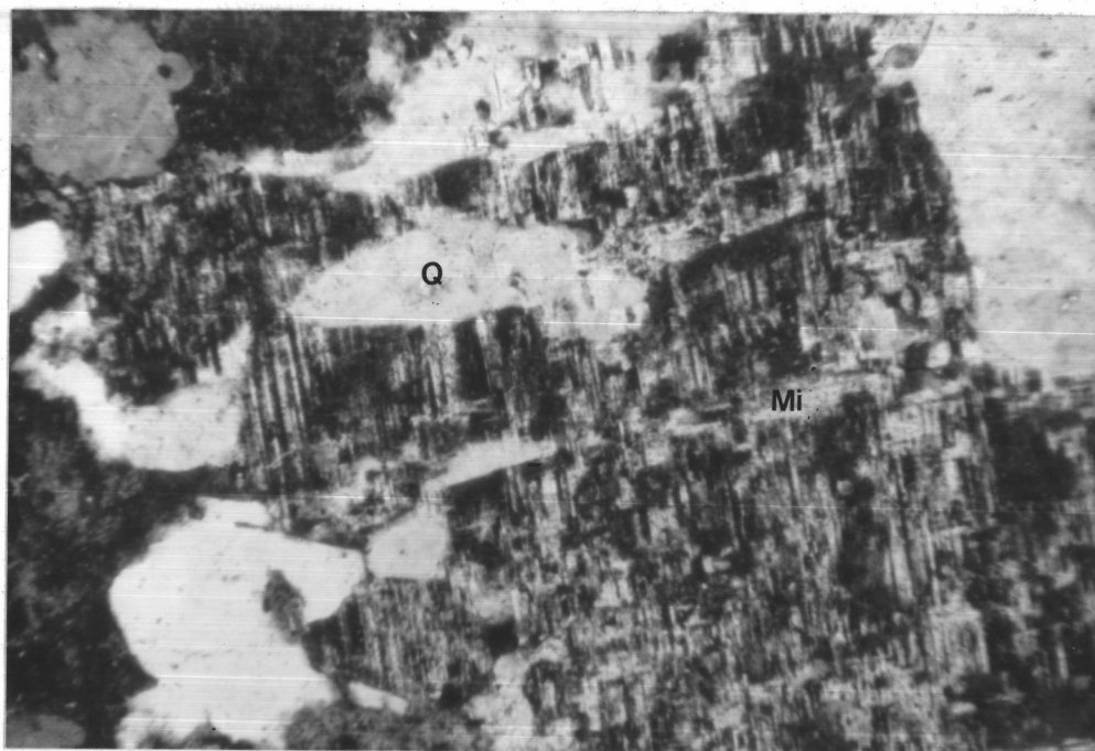
Fig. 3.7 Photomicrograph of granite in Phai Sali area showing perthitic microcline (Mi) which containing micrographic quartz (Q) (X-nicols, 45x).
