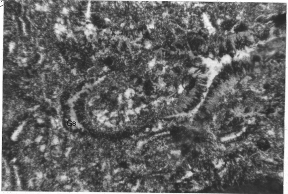
Fig. 3.24 Photomicrograph of rhyolitic tuff in Uthai Thani area showing the devitrification of glass shard (Gs) (X-nicols, 90x).
