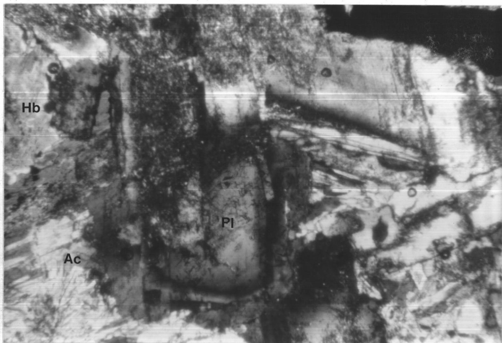
Fig. 3.2 Photomicrograph of diorite showing normal zoned plagioclase (Pl) associated with hornblende (Hb). Some of plagioclase grains are altered to sericite. The secondary amphibole is actinolite (Ac) (X-nicol, 45x).
