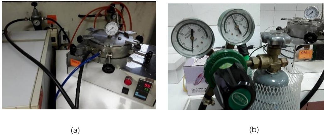
Figure 5 (a) pressure cooker connected with air pump (b) pressure cooker connected with nitrogen gas
