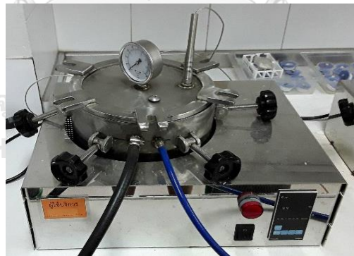
Figure 4 Pressure cooker with pressure release valve on the top surface of the lid. The temperature control panel is on the front side of the set up.
