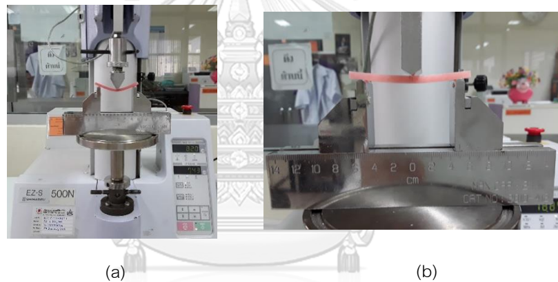
Figure 6 (a) lay the flat surface symmetrically on the supports of the flexural test rig (b) flexural strength test, using 3-point loading universal testing machine
