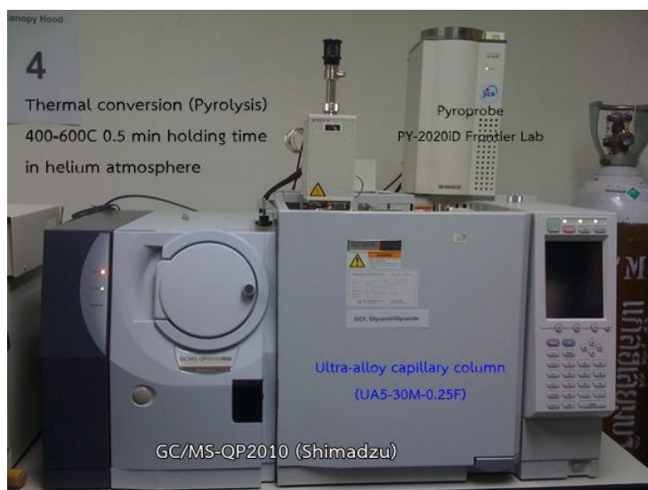
Figure 3.6 Pyroprobe GC/MS for pyrolysis reaction
