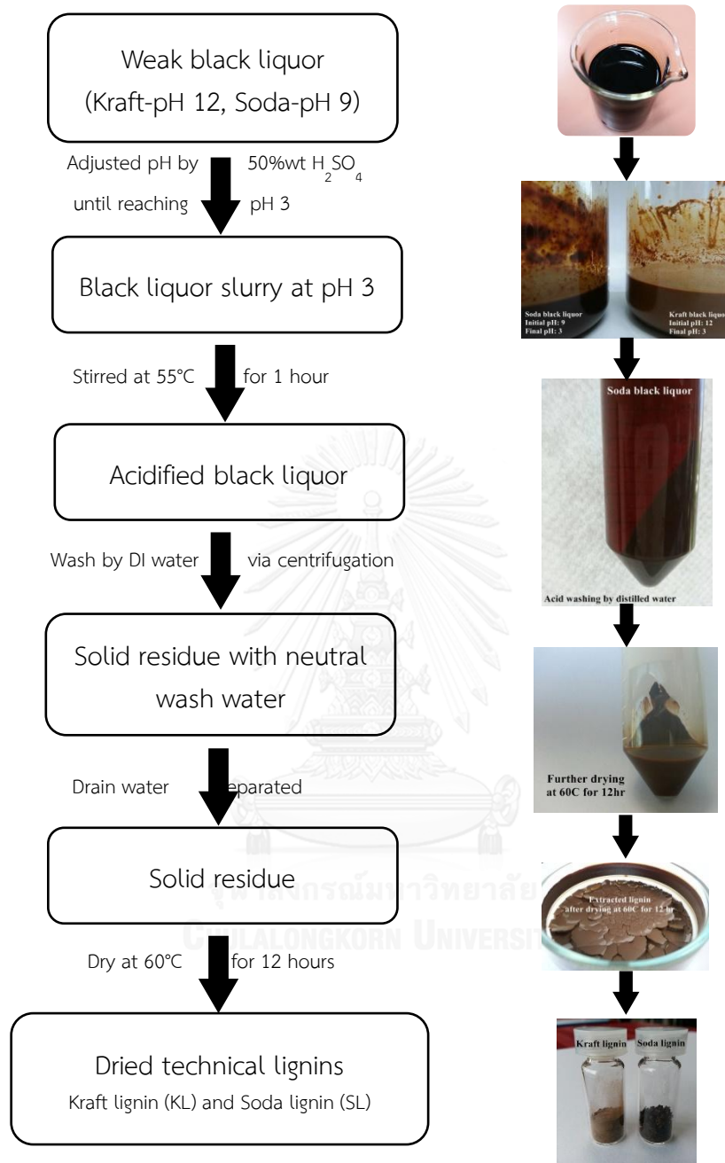
Figure 3.2 Acid precipitation for technical lignin from black liquor (adapted from Hu et al. (2013))
