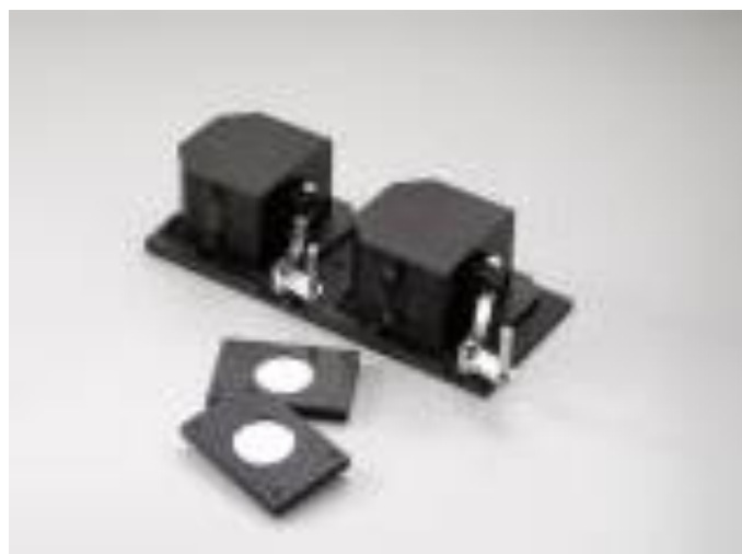
Fig. 3.5 As-synthesized powder in sample holder for UV-Vis diffuse reflectance analysis.
