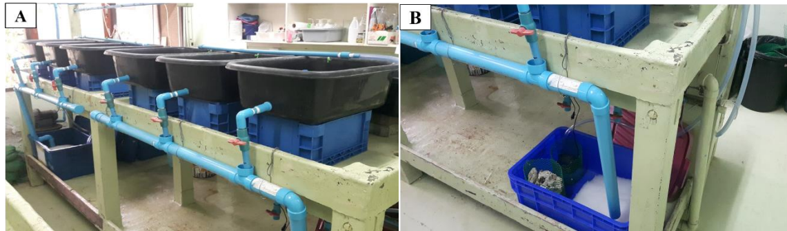
Figure 8 Culturing system A) the overall of the culturing system B) the storage plastic tank
