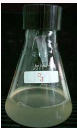
Figure 3.1 Erlenmeyer flask with the Eppendorf tube suspended at the top of the flask used for enrichment cultures.
