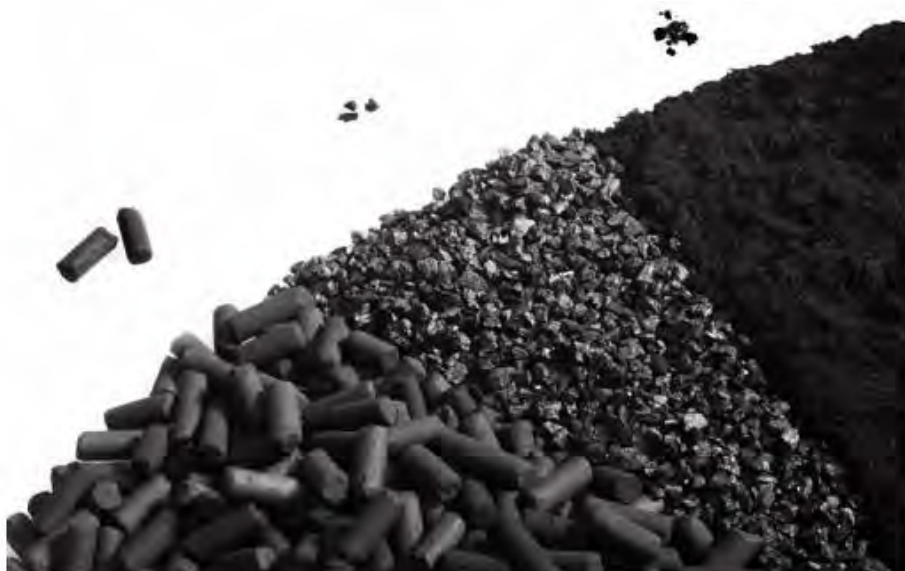
Figure 2.9 Pelleted, granular, and powder activated carbon (from left to right) ( www.redwhitechem.com ).
