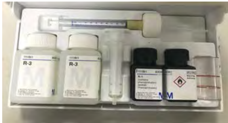
Figure 2.15 a titration kit, consists of a dropper syringe, R-1 and R-2 indicator, R-3 acid solution and sample syringe.
