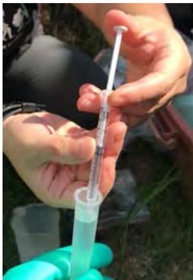
Figure 2.5 Collect samples for measuring silica, dilute with DI water 9:1
