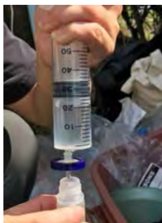
Figure 2.6 Collect samples for measuring \delta^{18}\text{O} and \delta\text{D} using 0.2-micron filter
