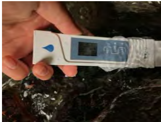
Figure 2.4 Measuring temperature and conductivity
