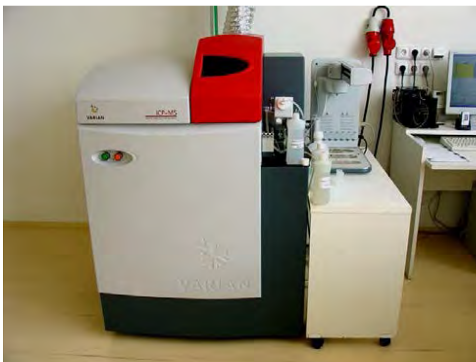
Figure 2.12 Inductively coupled plasma mass spectrometry (ICP-MS)
