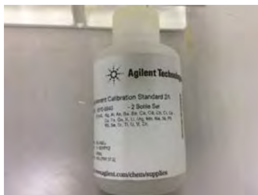
Figure 2.10 Mix standard solution for ICPMS
