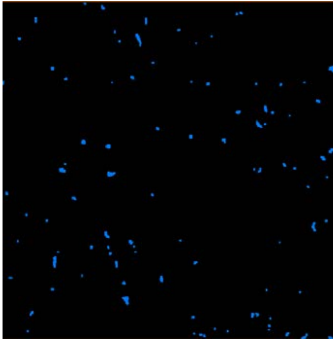
Figure 3.7 The binary image where one of the intensity levels equal to pore and one equal to the matrix in pore detection
