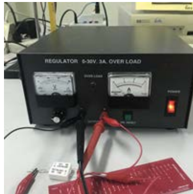
Figure 3.4: The regulator supplies the current to the Helmholtz coil
