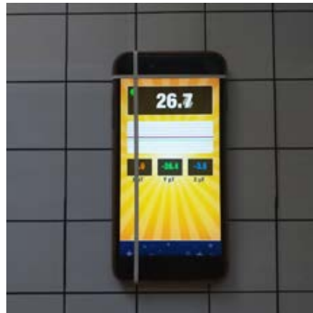
Figure 3.15: Measuring the magnetic field due to magnets on the plane
