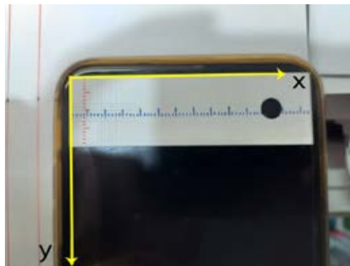
Figure 3.7: The area on the smartphone which is used to locate the sensor position
