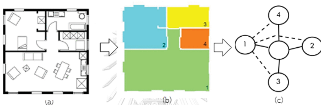
Figure 5: (a) is an original floor plan, (b) is the room layout segmentation of (a), and (c) is the topology graph of (a).
