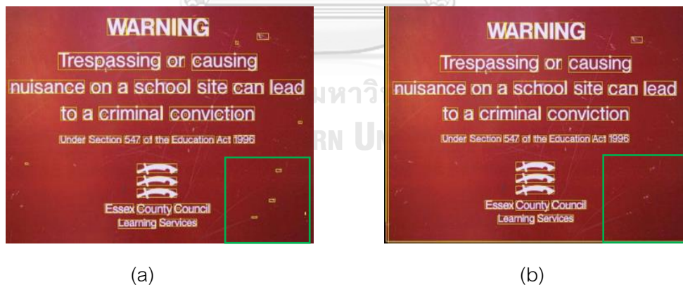
Figure 3.6 (a) The result after using 8 neighbor connected component to find bounding boxes, (b) the result after deleting bounding boxes that have area smaller than 250 pixels.
