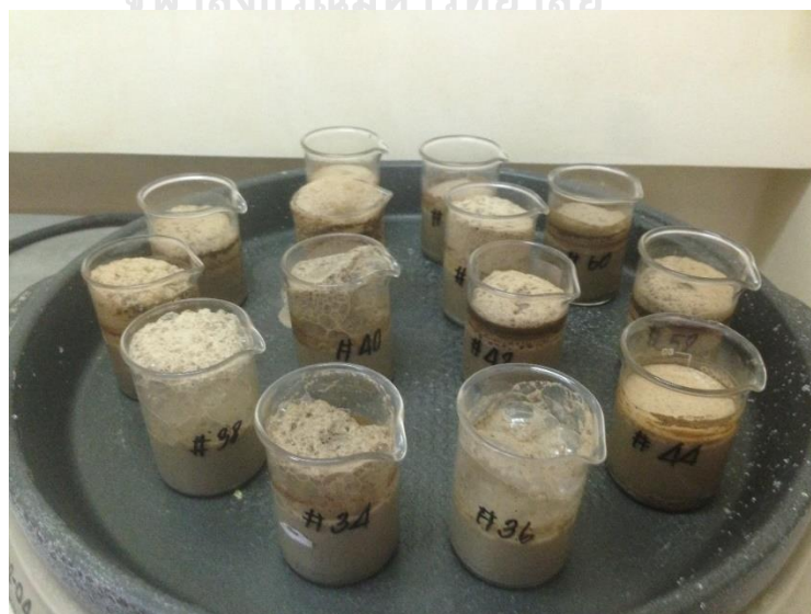
Figure 13 Organic content elimination in sample by H 2 O 2
