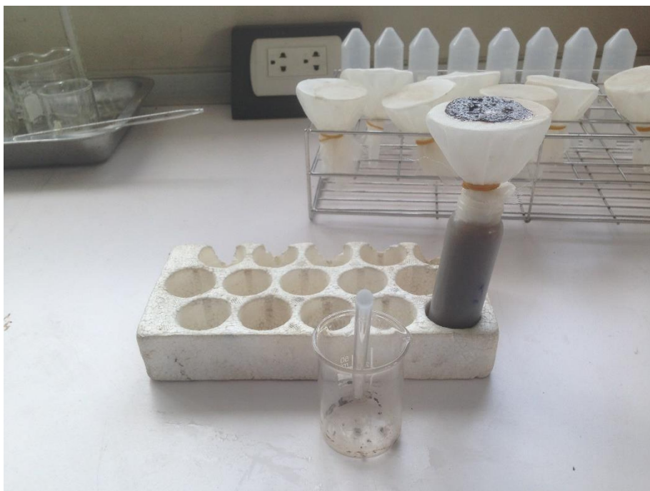
Figure 15 A sample was sieve with 0.2 mm mesh size
