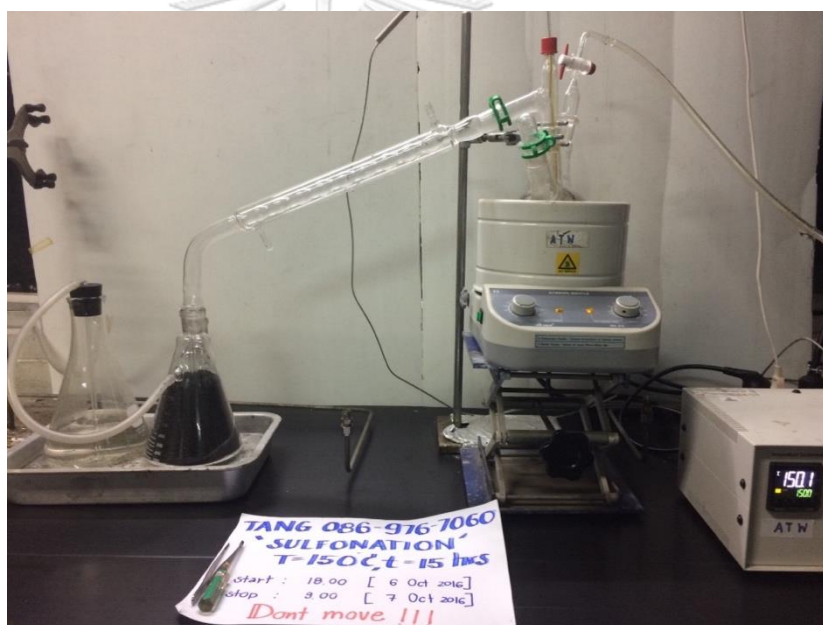
Figure 3.2 The set-up experiment for sulfonation
