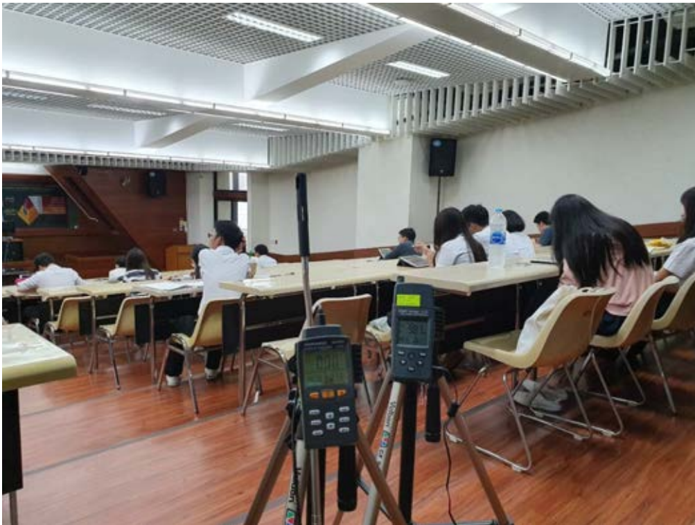
Figure 3.4 TM-4002 and SIRIUS ST-501 measuring indoor air quality parameters in the middle of the class in classroom 201 at Mahamakut building
