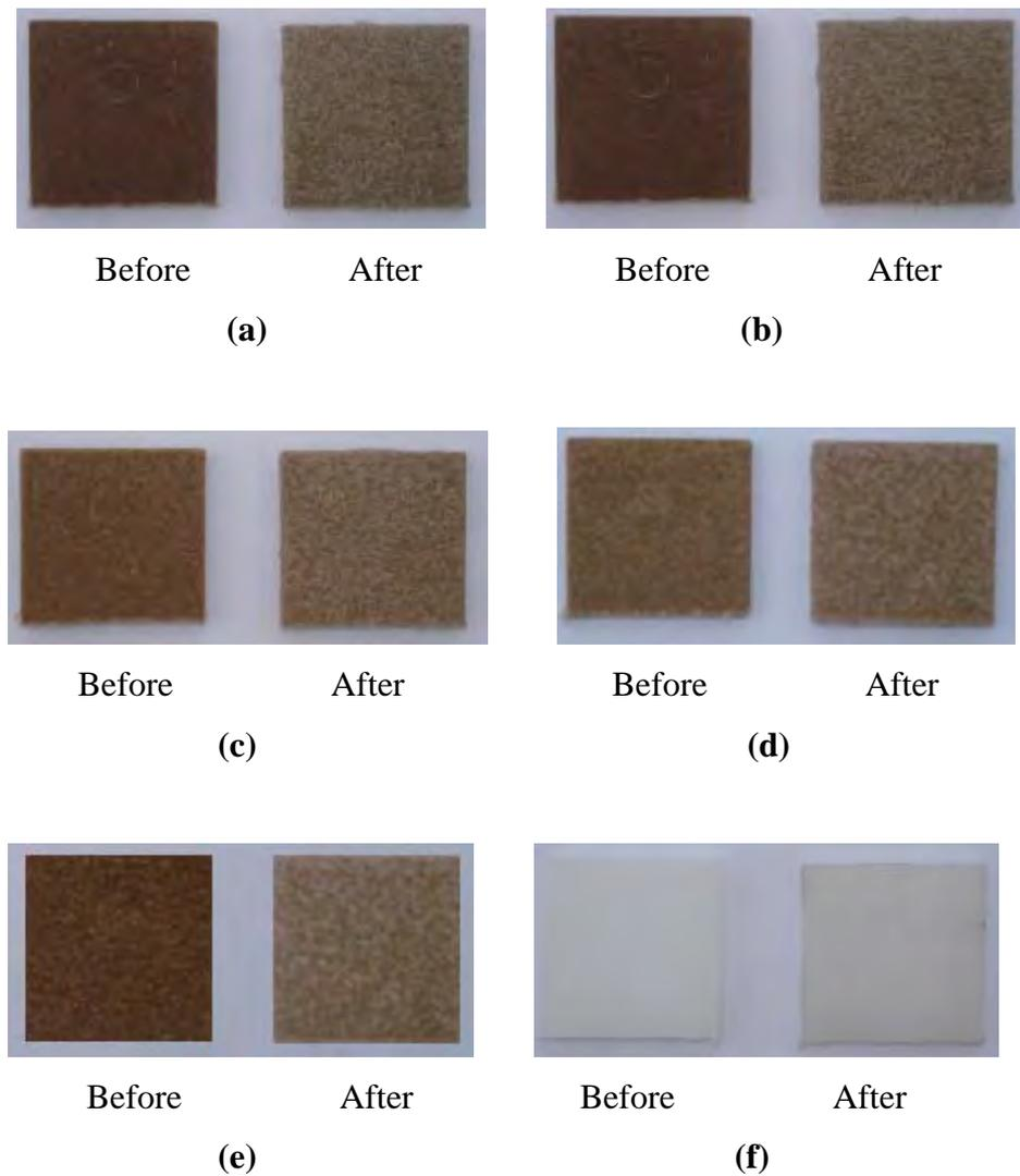
**Figure 5.25** Visual appearances of the HDPE/RH composites at 40% by weight, (a) 75 $\mu\text{m}$ , (b) 180 $\mu\text{m}$ , (c) 250 $\mu\text{m}$ , (d) 355 $\mu\text{m}$ , (e) 500 $\mu\text{m}$ , (f) pure HDPE before and after natural UV-weathering testing for 60 days.
