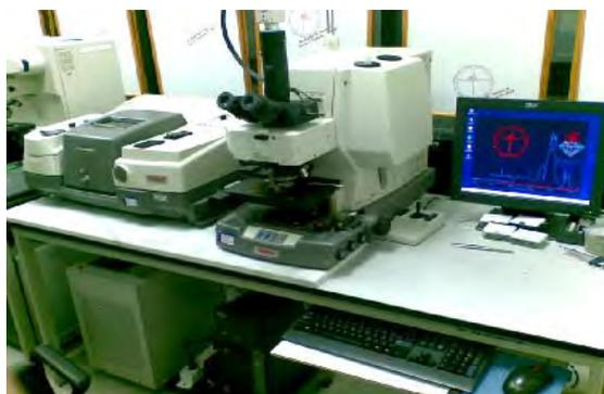
**Figure 4.15** Attenuated total reflectance (ATR-IR)
