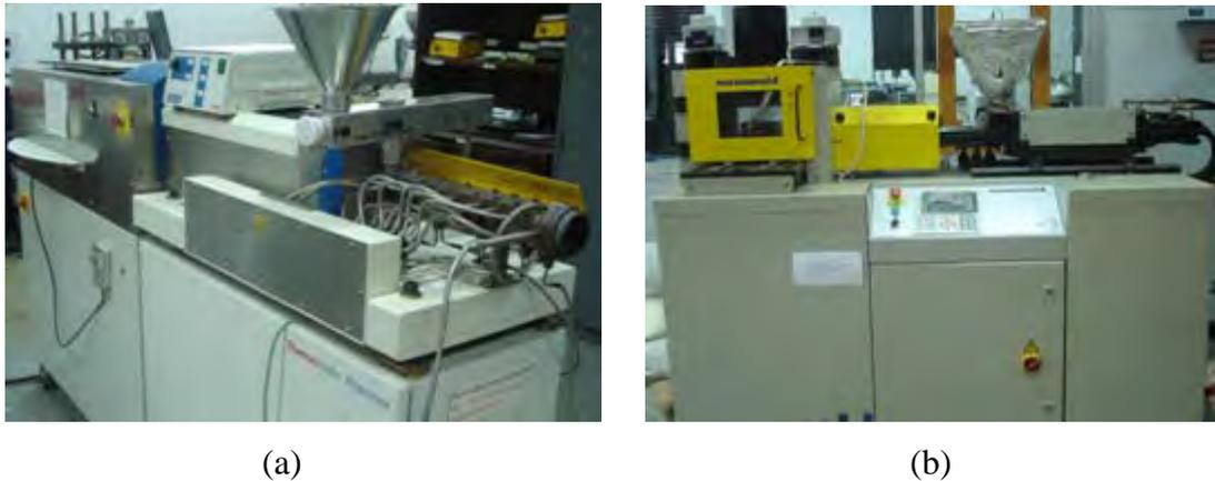
**Figure 4.3** (a) Twin screw extruder and (b) Injection molding.
