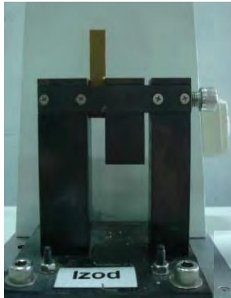
**Figure 4.6** Notched Izod impact test specimen.
