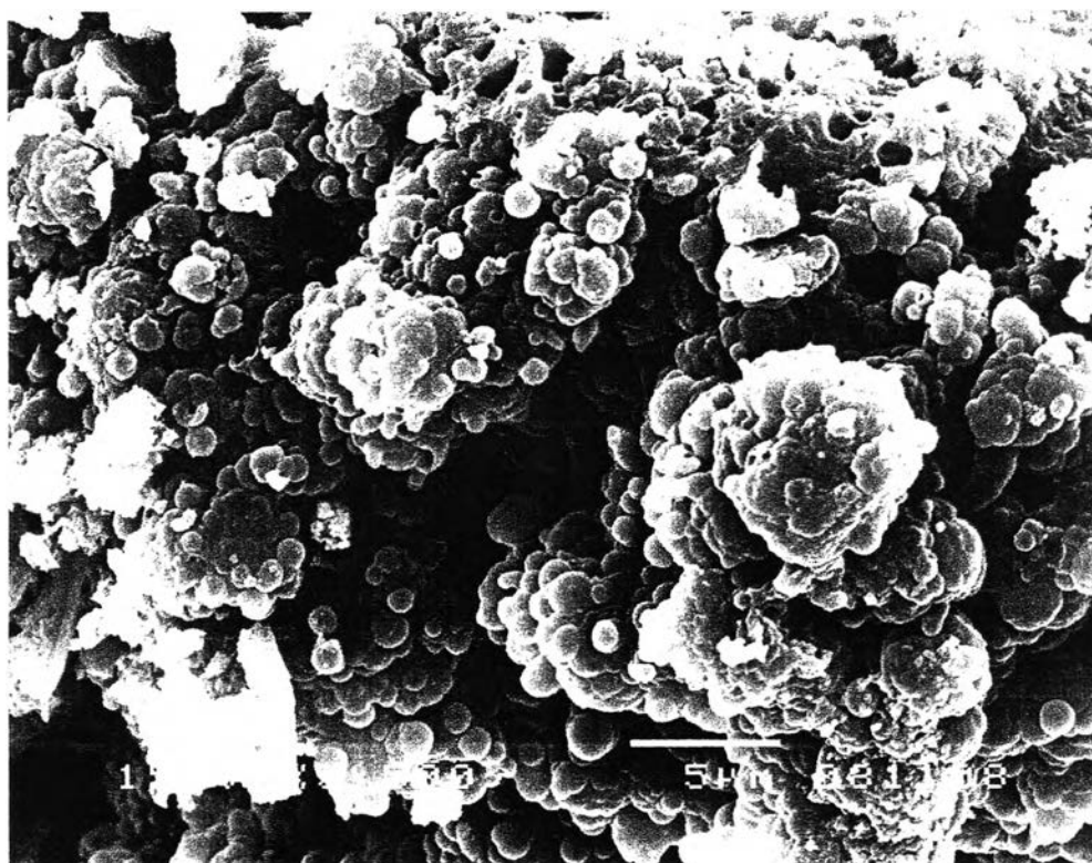
Figure 4.30 Scanning electron micrograph of the coated admicelled rubber (with 500 mM PPy) by using electrochemical method; magnification 1,500/15 kV.
