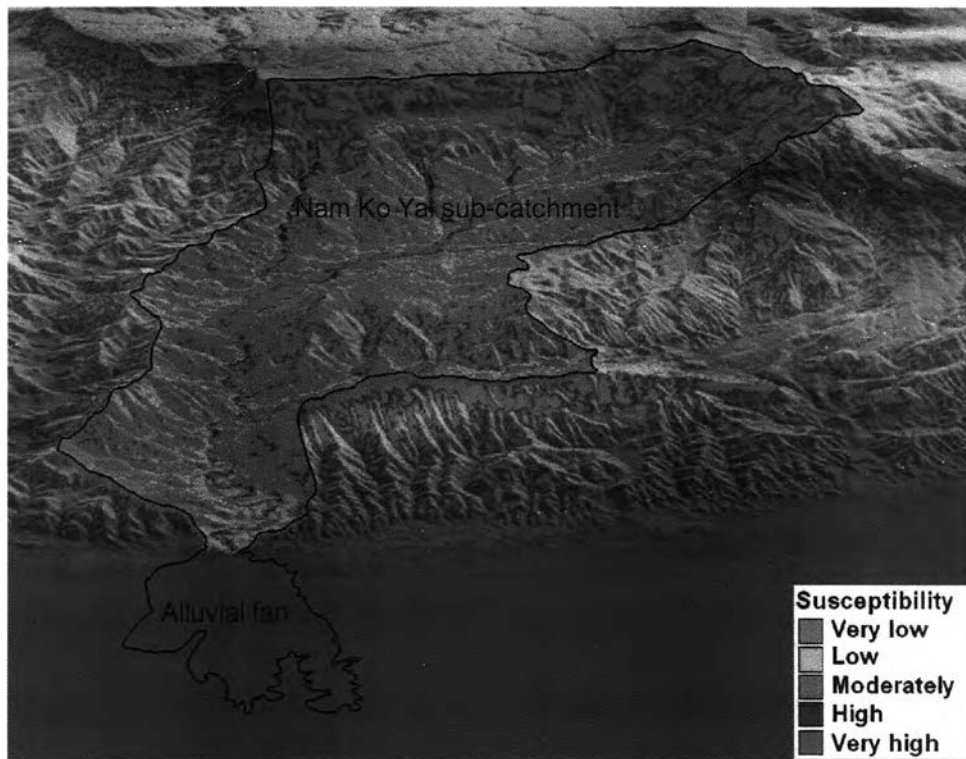
Figure 7-2 Three-dimensional drupe of five classes susceptibility of very high, high, moderate, low, and very low, through a 1:20,000 base-scale DEM in Nam Ko Yai sub-catchment. Very high to very low susceptibility was noted here.
