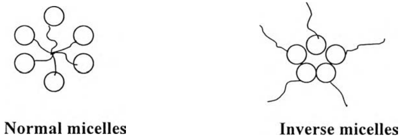
Figure 2.2 Schematic diagram of normal micelles and inverse micelles
